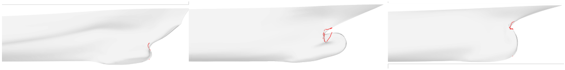
Figure 8.26: Examples of invalid (self-intersecting) designs resulted from the GAN model. The red curve indicates the regions of intersection.
