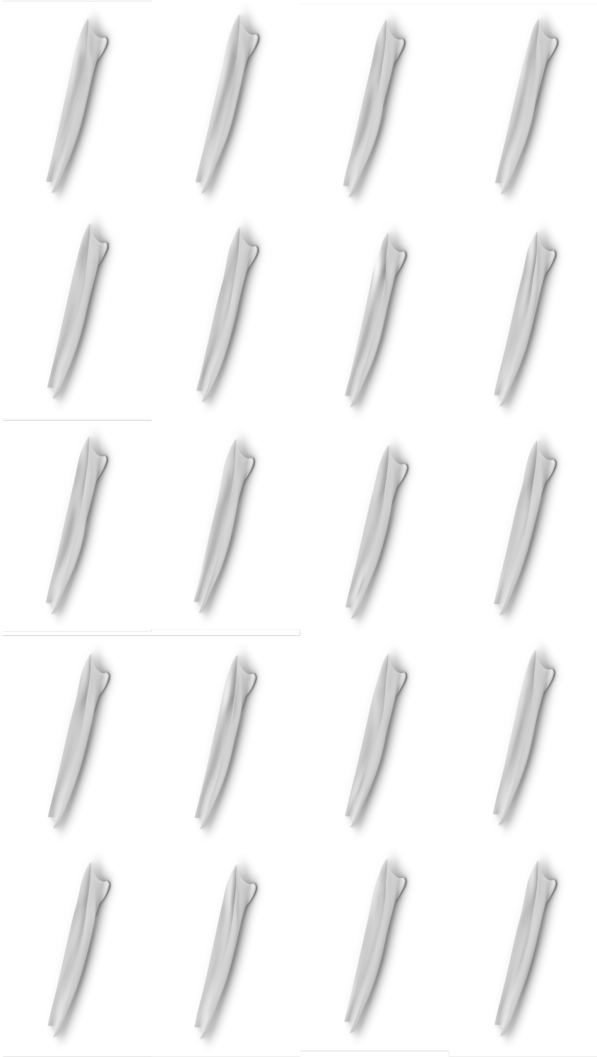
Figure 8.6: Some of the synthetic design variation of DTMB hull in Fig. 8.4 created for training ShipGAN.
