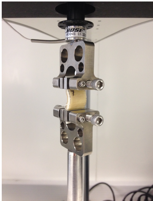
Figure 3.4: 25mm grips of Bose 3200 testing instrument
