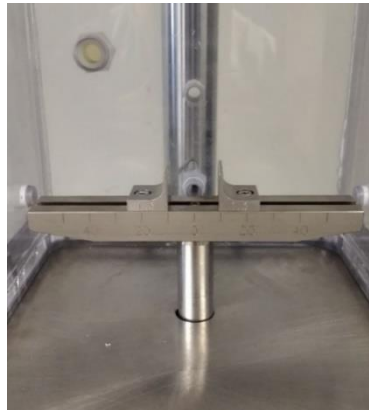
Figure 4-17 Support podium mounted onto the water bath rod.
