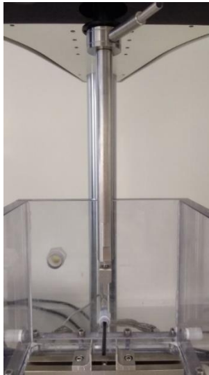
Figure 4-18 Attaching the deflection bar (indenter) to the load cell using the attachment rod.
