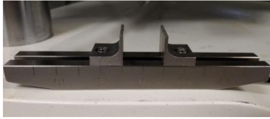
Figure 4-16 Supports with a diameter of curvature of 1.3mm placed onto the support podium.
