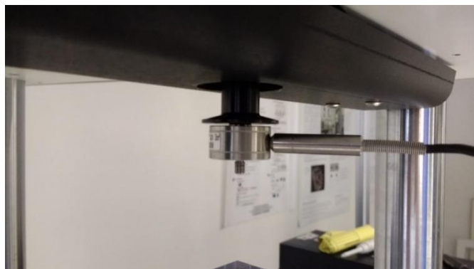
Figure 4-15 The 450N load cell attached to the moveable crosshead.
