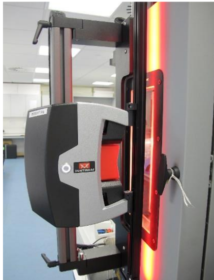
Figure 4-2 Video extensometer mounted on the environmental chamber door
