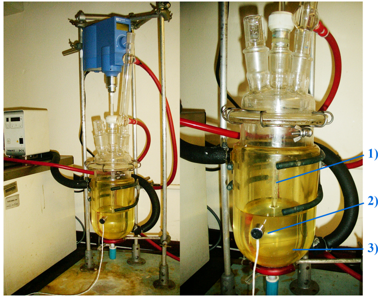
Figure 3.1: Reactor vessel. 1: Stirrer 2: Transducer 3: Oil Jacket
