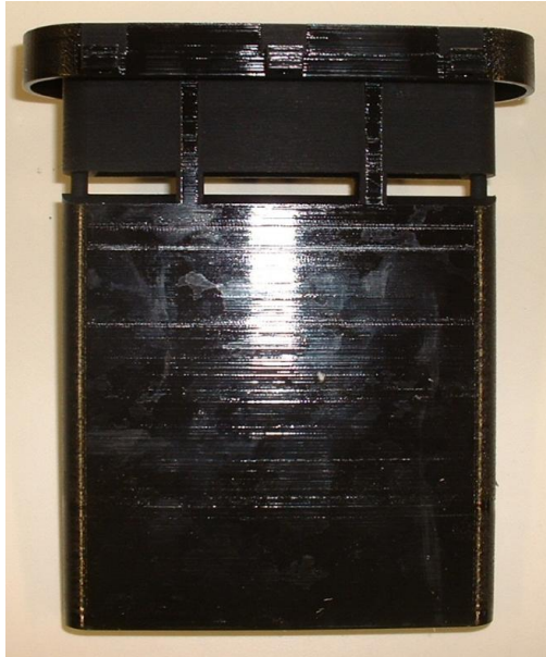
Figure 246: Rapid prototyped Mark II sparger.
