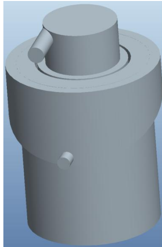
Figure 206: A proEngineer model of a fluid path based upon the dimensions of a Medos Hilite 800LT pediatric oxygenator.
