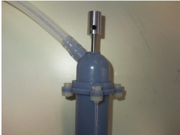
Figure 85: Picture showing the coupling between the pump and the motor.
