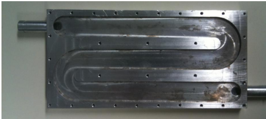
Figure 185: Mark II Heat exchanger cut in aluminium.
