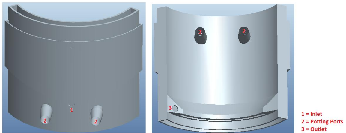
Figure 224: ProEngineer model of the oxygenator main body.
