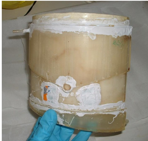
Figure 230: Rapid prototyped oxygenator potted and sealed ready for use in the lab.
