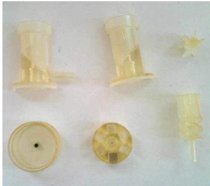
Figure 326: Picture showing a selection of rapid prototype parts used to make the magnetically coupled direct drive axial flow blood pump.
