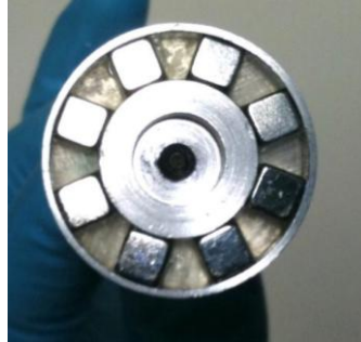
Figure 325: Picture of an impeller shaft cut from aluminium with magnets, spacers and male diamond bearing in the base.
