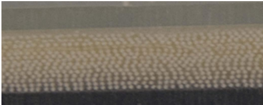
Figure 212: Picture showing fibers within a rapid prototyped oxygenator module, prior to the fibers being opened.
