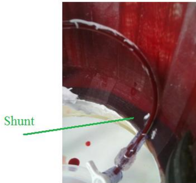
Figure 235: A picture of bright oxygenated blood next to dark un-oxygenated blood in the main casing confirming the presence of flow shunting in the oxygenator module.
