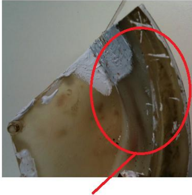
Area in which the heat exchanger has bowed
