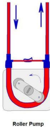
Figure 14: Diagram of a double head roller pump (taken from media.photobucket.com).
