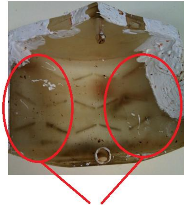
Areas in which the heat exchanger has bowed
