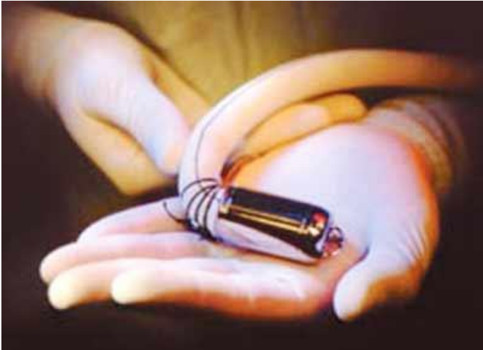
Figure 21: Jarvik 2000 implantable left ventricle assist system (Taken from www.asaio.com ).
