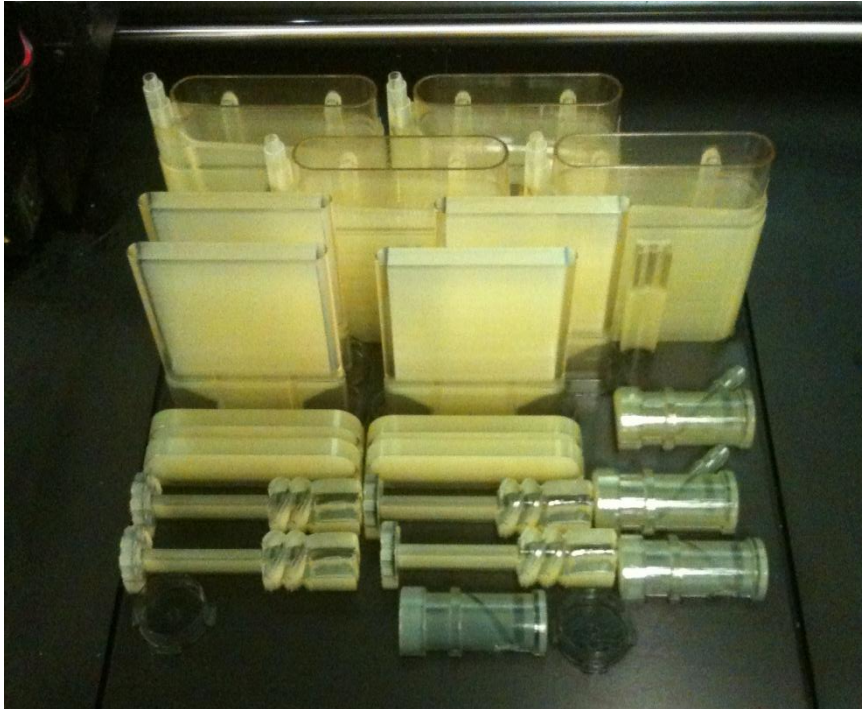
Figure 82: Rapid prototyped parts in the Objet machine after printing prior to being cleaned and processed.
