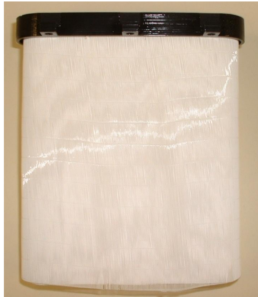
Figure 247: Mark II sparger with hollow fiber membrane mat wrapped around it.
