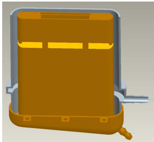
Figure 249: ProEngineer of the sparger within the main casing after the top has been removed to leave the sparger “floating” in the main casing supported by potting compound.
