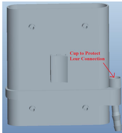
Figure 286: ProEngineer model showing the location of the bubble trap on the oxygenator casing with a leir connection protection cup which is highlighted.
