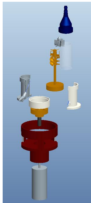
Figure 324: Exploded view of the magnetically coupled direct drive concept.
