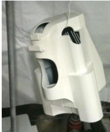
Figure 303: Picture of the rapid prototyped casing being sprayed in the paint bay.
