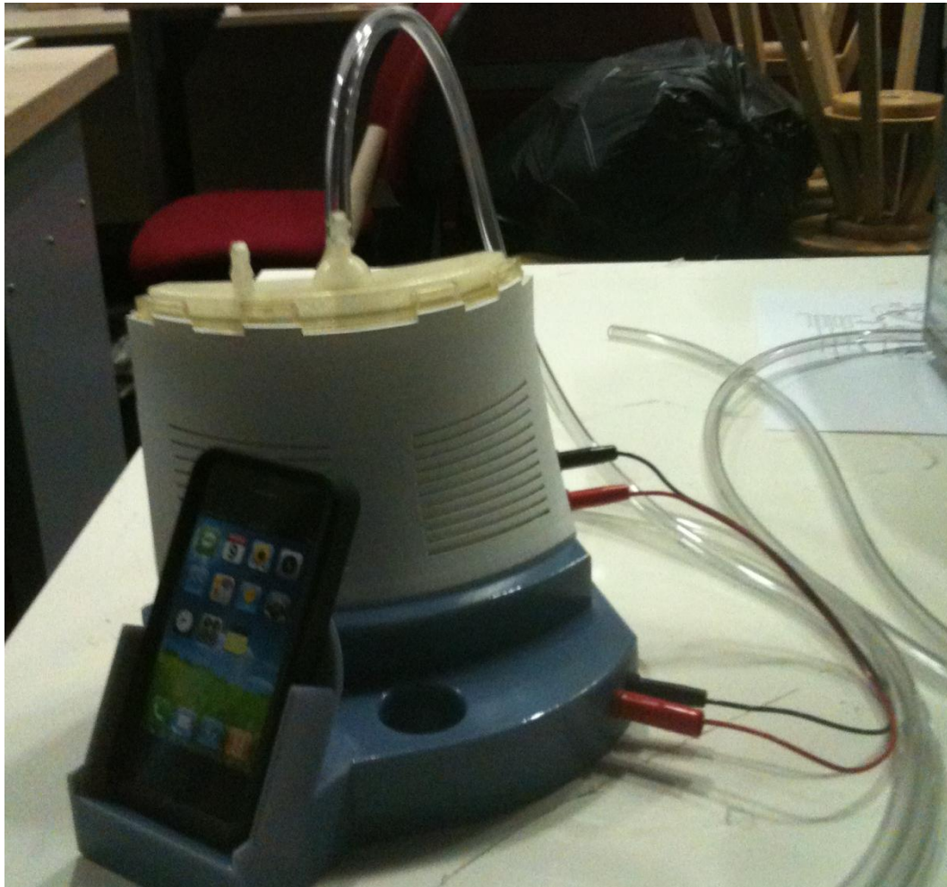
Figure 70: Rapid prototype of concept 3 with a holder and example control device and connections.
