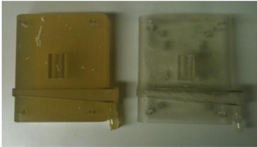
Figure 83: Comparison of rapid prototyped parts with and without support material.
