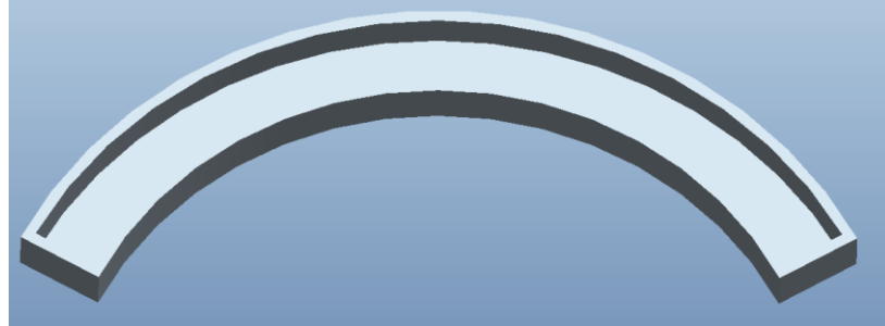
Figure 227: ProEngineer model of the potting cap used to prevent leakage of compound during the potting process.
