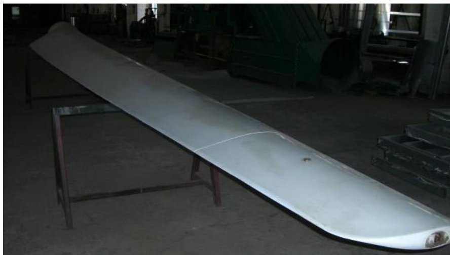
Figure C1: Detached 9.8 m wind turbine blade
