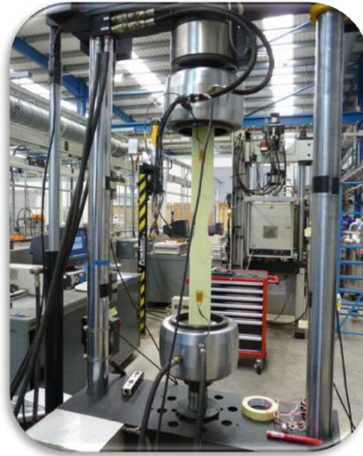
Figure B16: Instron 8508 Tensile loading machine gripping a waisted GFRP coupon
