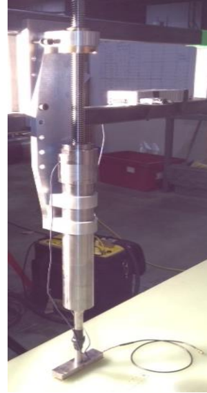
Figure 5.38: MFC bonded to GFRP sample using flexible load manipulator
