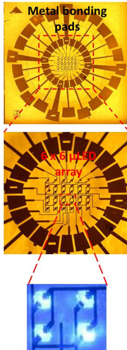
Figure 2.20: a), b) Layout of the metal tracks for a 6x6 array of \mu TP \mu LEDs. The \mu LEDs are printed within the dashed red box. c) A close-up photograph of the \mu LED array printed on glass. Each \mu LED is 100 \times 100 \mu\text{m}^2 .
