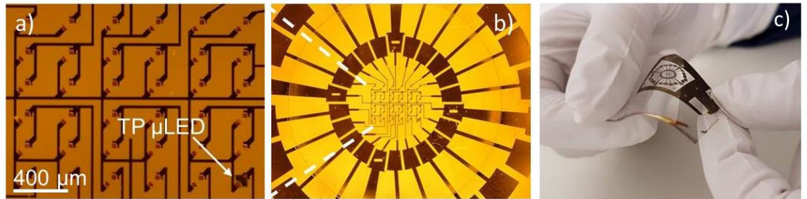
Figure 1: A single \mu LED micro-transfer printed onto 30 \mu m-thick mechanically flexible glass.
