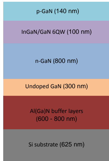
Figure 2.9: Schematic of the as-grown GaN-on-Si wafer used for suspended \mu LED fabrication.
