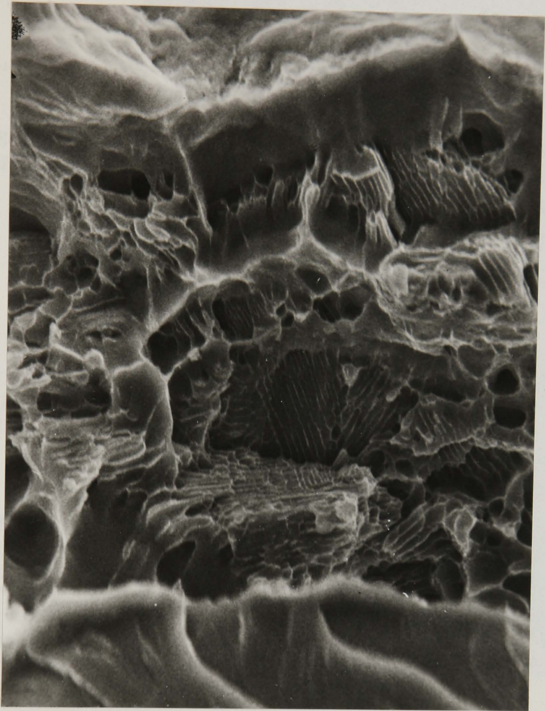
FIGURE 31 (c) : SCANNING ELECTRON MICROGRAPH OF FRACTURE SURFACE PRODUCED DURING C.O.D. TEST ON ALLOY P8 AT -77^{\circ}\text{C} . THE MICROGRAPH ILLUSTRATES THE MIXED CLEAVAGE-DUCTILE FAILURE MODE.
