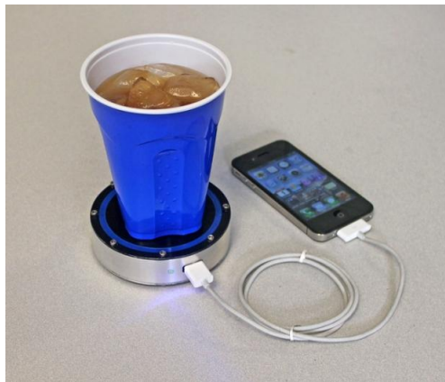
Figure 4.3: Making use of temperature differences in gadgets; exploiting ice beverage and ambient temperatures in order to induce electrical energy to charge phone. (taken from www.tweaktown.com )
