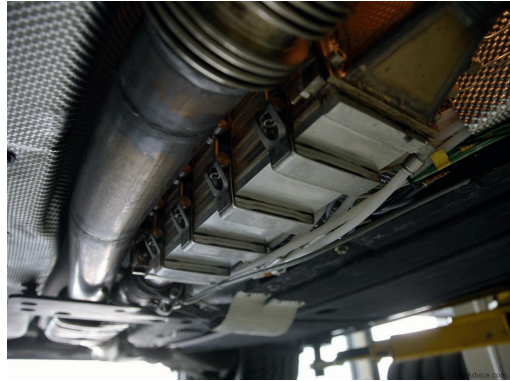
Figure 4.2: Thermoelectric generator applied in automobiles; to capture waste heat and convert into electrical energy which can be used to power other appliances. (taken from www.caradvice.com )
