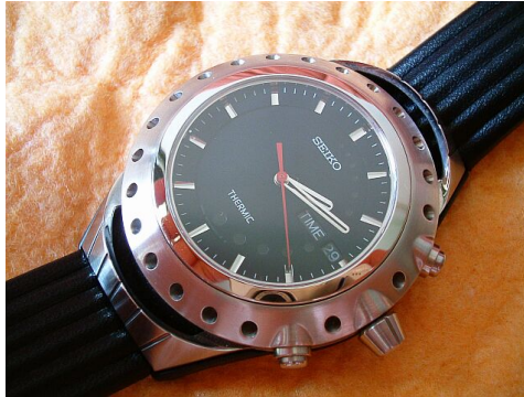
Figure 4.4: Thermoelectric element applied in wrist watches, making use of temperature differential between body heat and ambient temperature. (taken from www.ecofriend.com )
