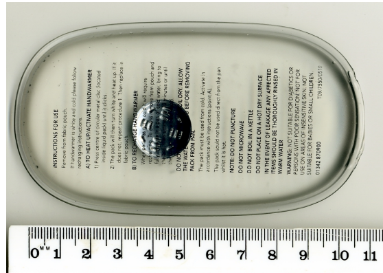
Figure 4.12: Example of sodium acetate pocket warmer pouch (taken from Wikipedia)
