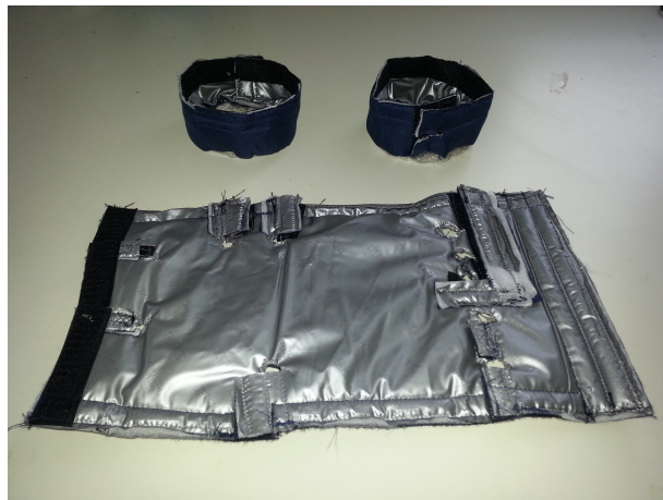
Figure 4.19: Finished Heat Exchanger Insulation (inside silver lining)
