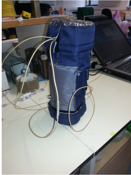
Figure 4.21: Assembled heat exchanger bag with insulation
