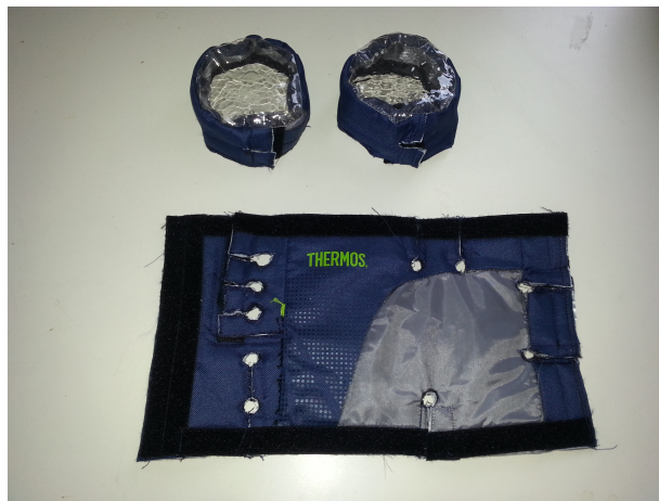
Figure 4.20: Finished Heat Exchanger Insulation (outside cover)
