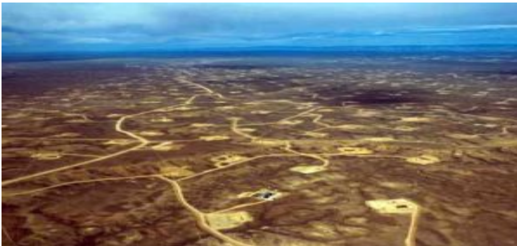
Figure B.2: Drilling Pads in West Virginia USA at a Density of One Well per Pad and 6 Pads per Square Kilometre.
