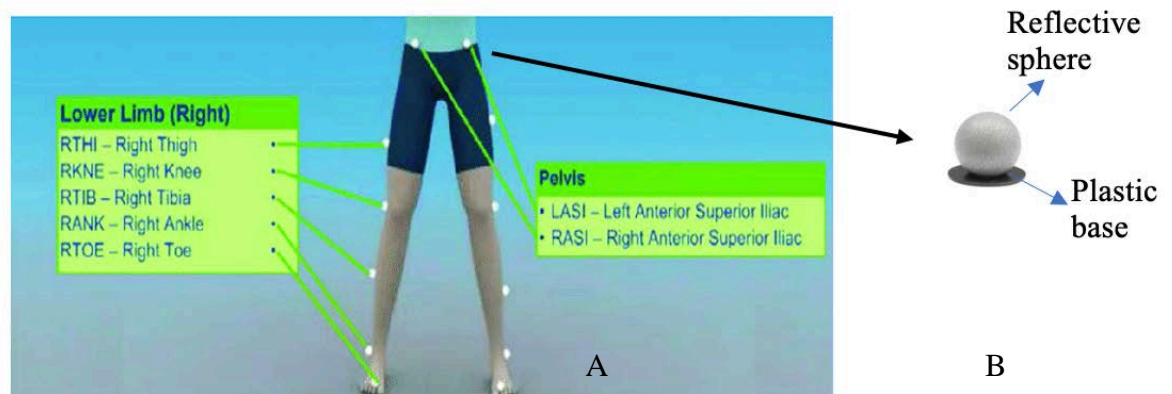
Figure 3-4 (A) The placement of the retro-reflective markers adapted from Vicon® 2010. (B) The reflective marker
