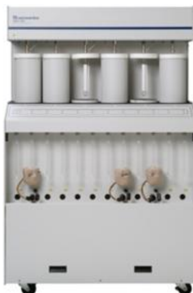
Figure 44 - Micromeritics ASAP 2420 Surface Area and Porosity Analyser. 341
