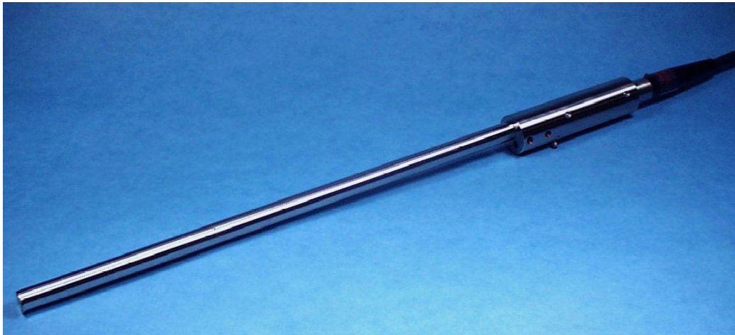
Figure 2.7. NIST probe with immersion sleeve based on the design of Carraba and Rauh (InPhotonics, USA) 105 .
