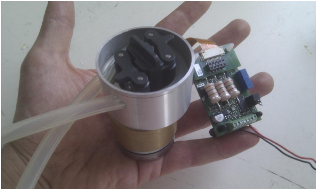
Figure 58 – Photo of roller pump prototype.
