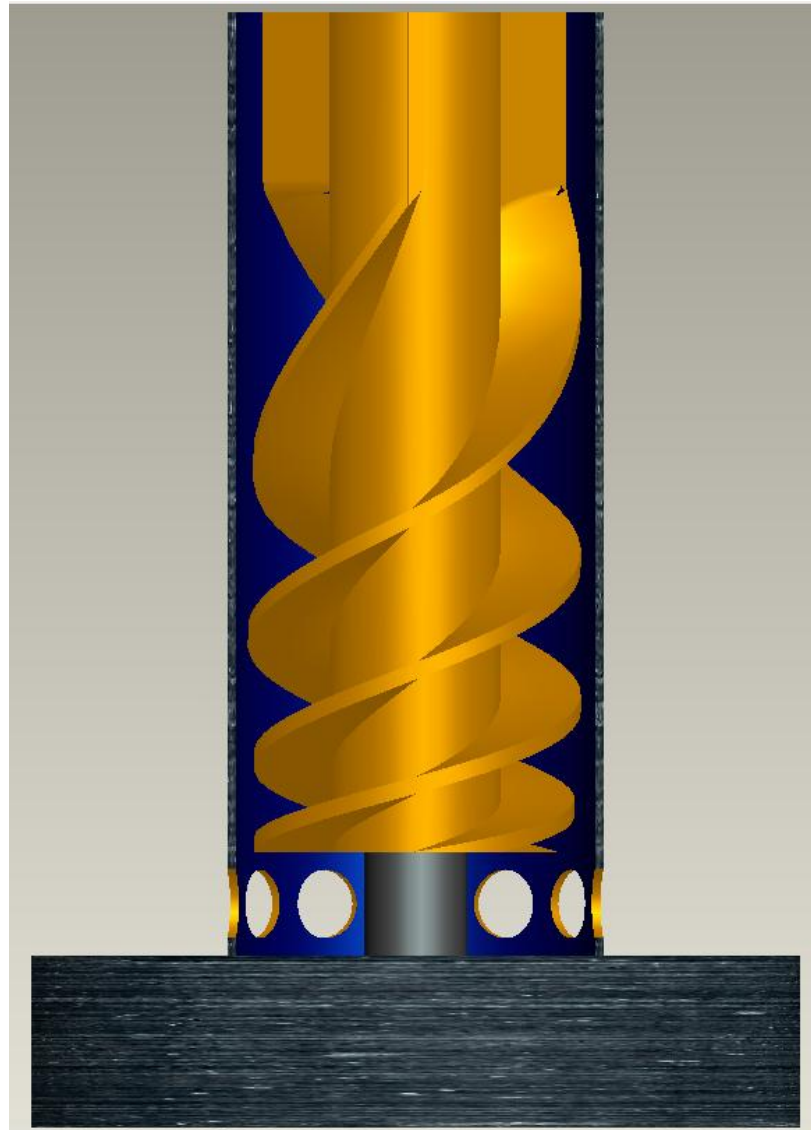
Figure 24 - Side view of an axial flow pump, utilising direct drive, displaying half-cut housing.
