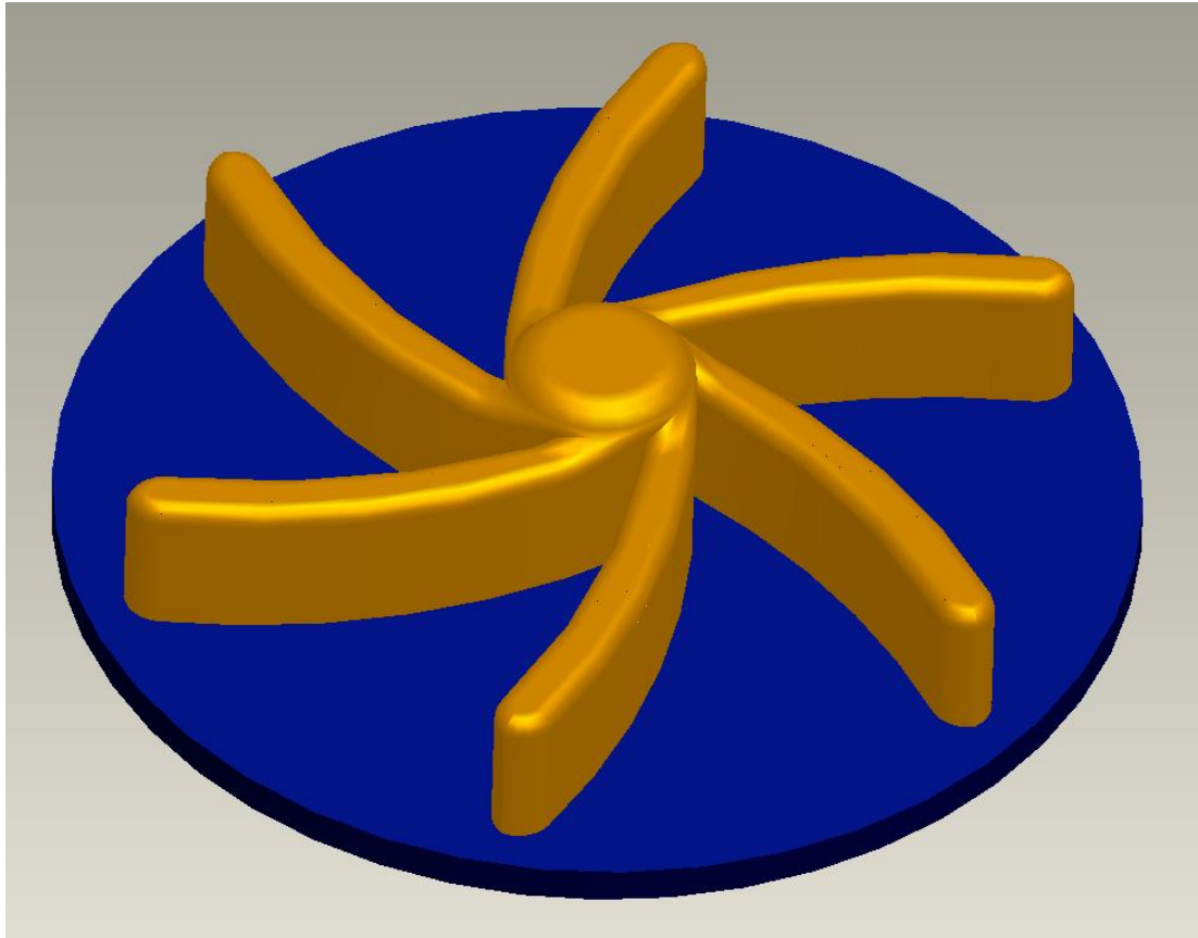
Figure 36 – Angled view of centrifugal impeller created in ProEngineer.
