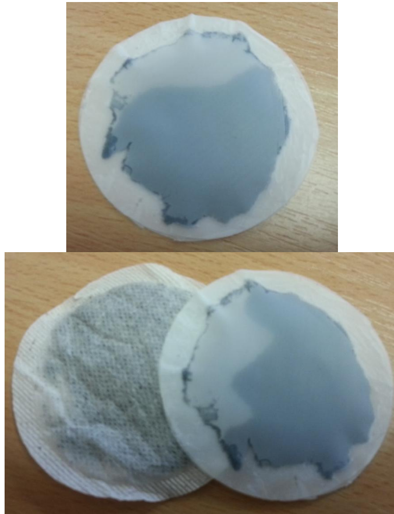
Figure 45 - Teabag configuration of immobilised adsorbent.
