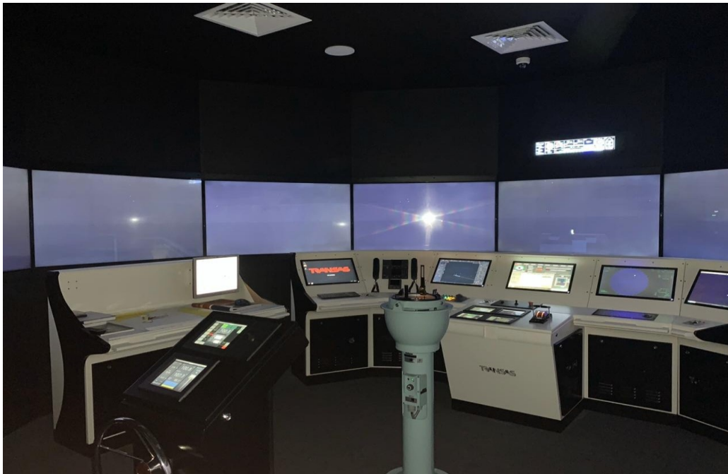
Figure 8.3 TRANSAS 270° full mission navigation bridge simulator
