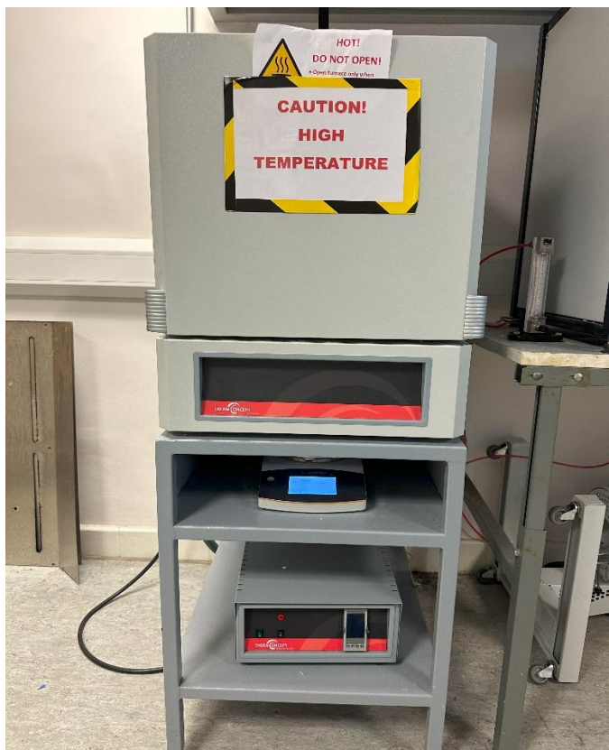
Figure 3.5: Calcination furnace-balance system
