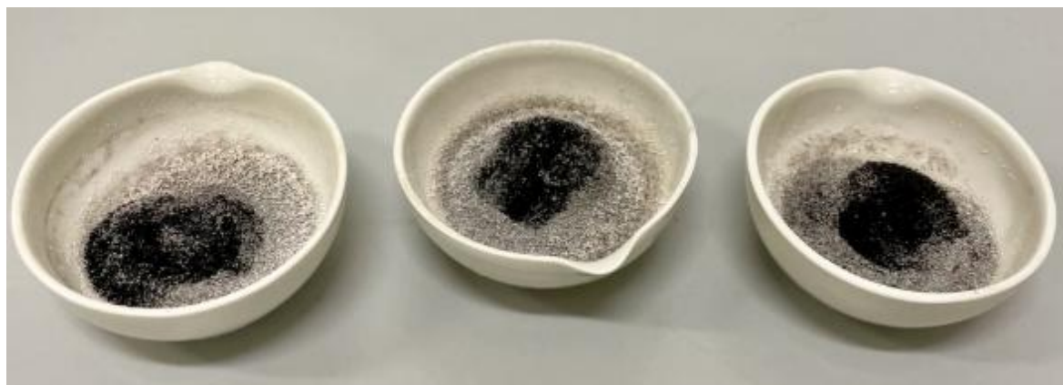
Figure 5.1: Calcined Kola nut pod husk catalysts A, B and C produced in this current research.
