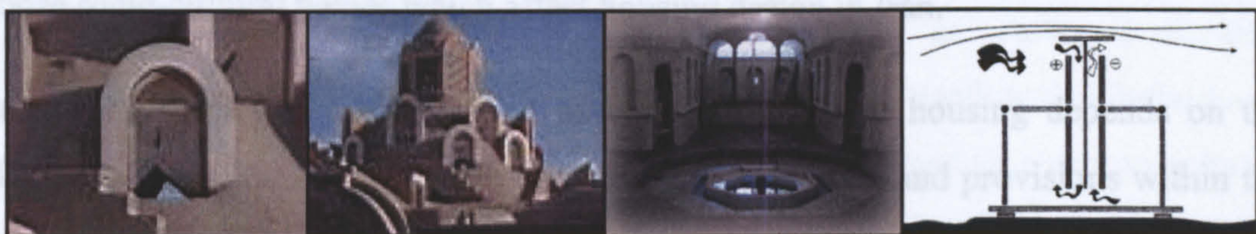
Figure 1. 18 Illustration of the Badgir and Howz-khaneh & schematic diagram of the badgir's function. Source: http://iranianarchitecture.20m.com/ & Battle McCarthy, 1999. P20.
