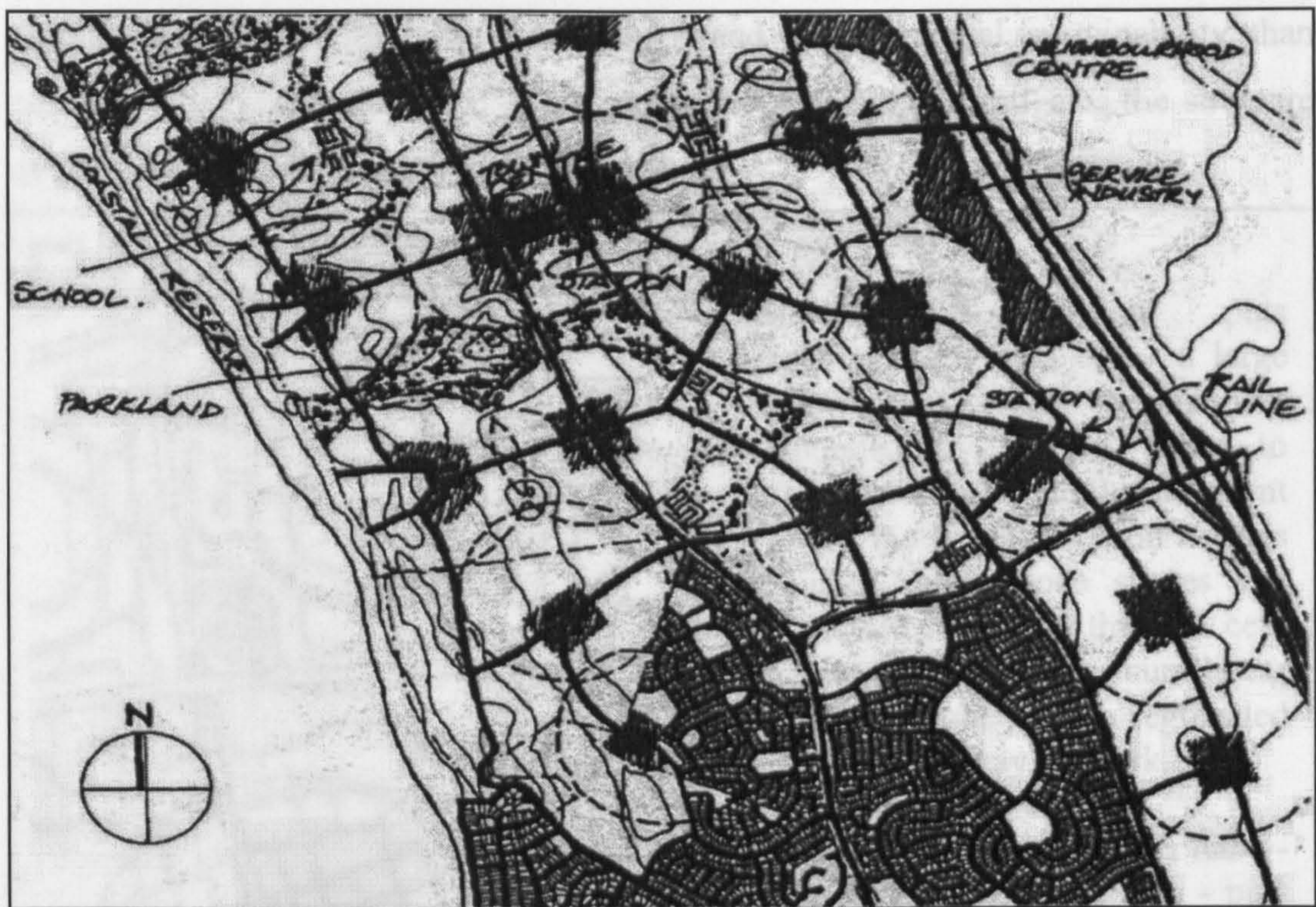
Figure 2. 2 Cluster of neighbourhoods that form a town and the location of neighbourhood and town centre at the intersection of major roads.
