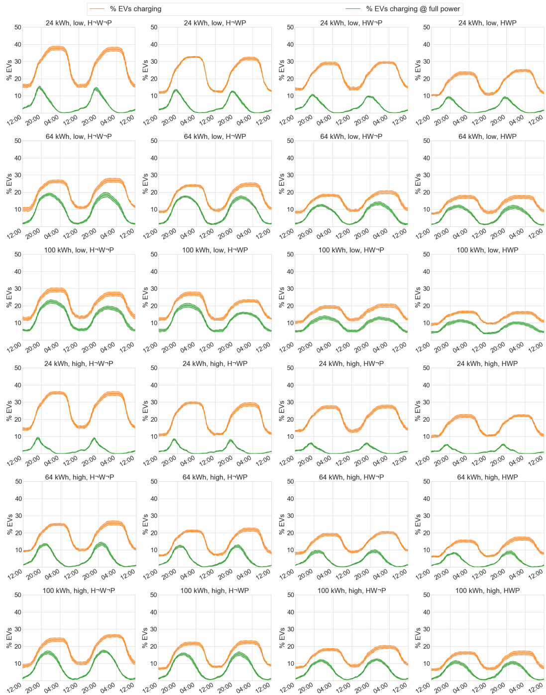
Figure 4.54: Coincidence of EVs charging and coincidence of EVs charging at full power for varying combinations of battery capacity, charger power and levels of access to charging at different locations
