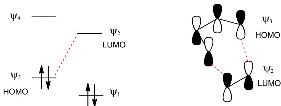
**Figure 3.1** – Interaction of the HOMO of the diene and the LUMO of the dienophile in the Diels-Alder cycloaddition
