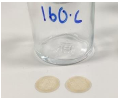
Figure 74 - Pure Affinisol™ Printed at 160°C
