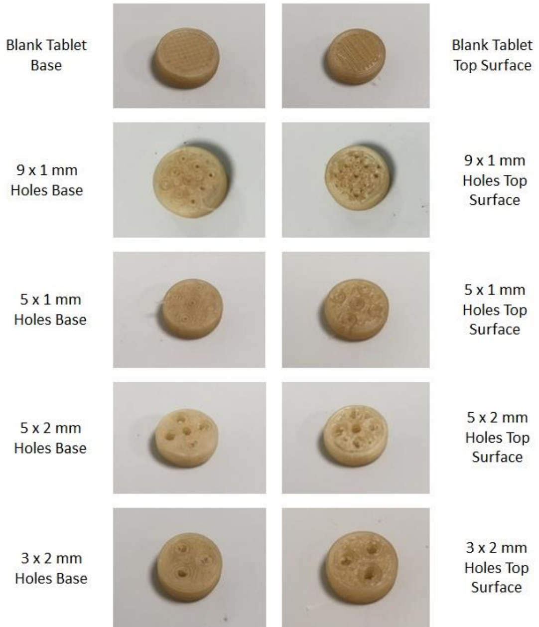
Figure 109 - Printed Tablets with Varying Holes Incorporated into the Design
