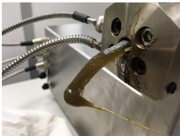
Figure 69 - Extrusion of Powdered PVA (13000-23000 MWt)
