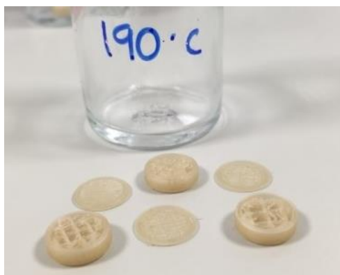
Figure 76 - Pure Affinisol™ Printed at 190°C
