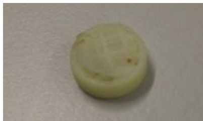
Figure 44 - PVA Tablet with Bottom Layers Peeling Away
