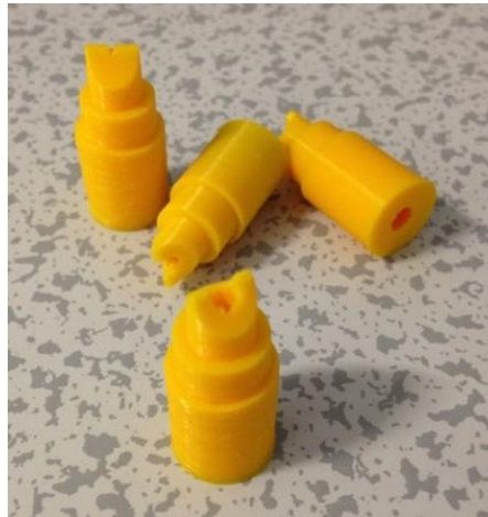
Figure 45 - New Flex Filament Adaptor with Correctly Positioned Hole
