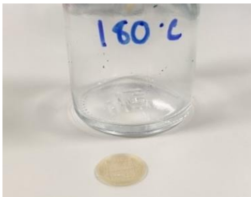
Figure 75 - Pure Affinisol™ Printed at 180°C
