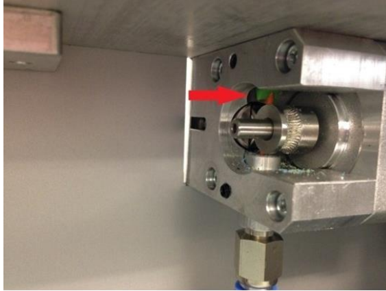
Figure 42 - Flex Filament Adaptor Fitted at the Printer Gear Wheel
