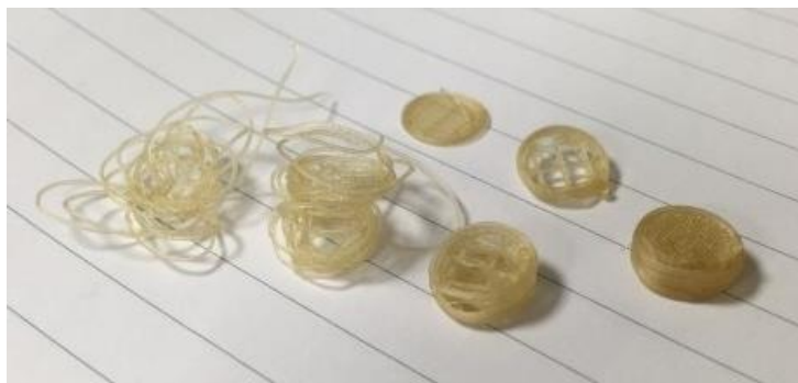
Figure 78 - Printing of DoE Formulation 2 (20% CAR 80% Affinisol™) 195°C print temperature.
