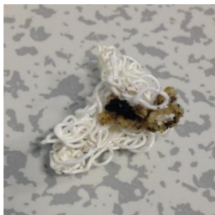
Figure 40 - Burned PVA removed from clogged printer nozzle
