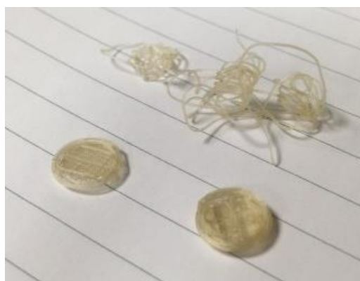
Figure 77 - Printing of DoE Formulation 1 (1% CAR 99% Affinisol™) 195°C print temperature.
