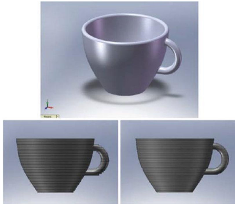
Figure 13 - Top - CAD drawing of a teacup Bottom - images showing printed teacup with differing layer thickness. 65
