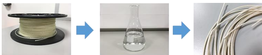
Figure 33 - Solution Loading Process. Left - Commercially available filament. Middle - A solution containing the desired API. Right - Drug loaded filaments after drying.
