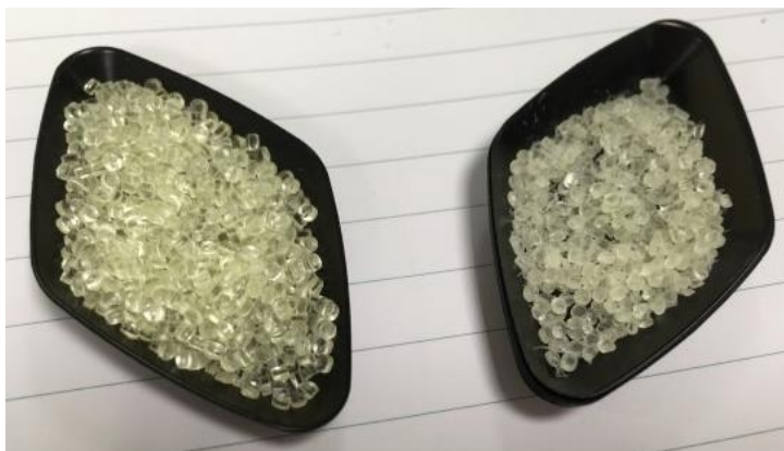
Figure 66 - Left - pelletised starting material Right - milled PVA using 2 mm holes
