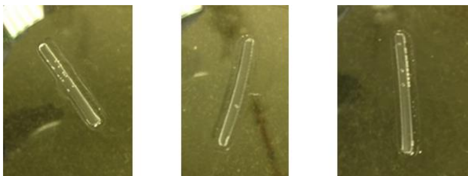
Figure 34 - Left - anisole, middle - butyl acetate, right - isobutyl acetate after filament removal
