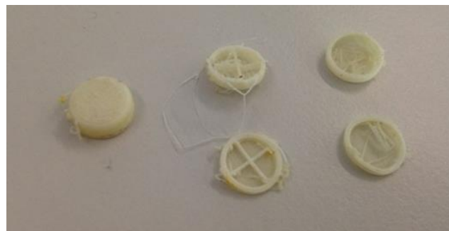
Figure 47 - PVA Placebo Tablets with 10% Infill
