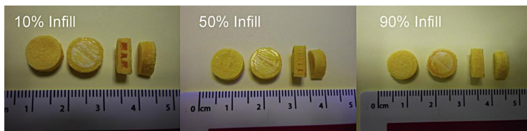
Figure 20 - Printed tablets with a view of cross-section. 80
