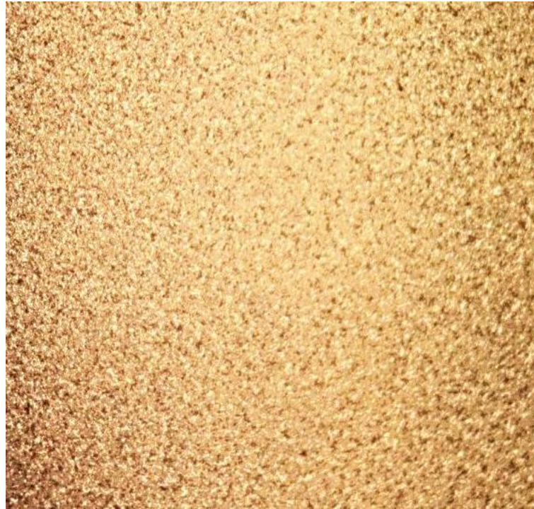
Figure 5.4. Undamaged fine lap diamond surface under 10x magnification.
