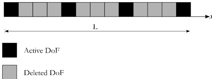
Figure 4-1: Schematic representation of 1D reduction process
