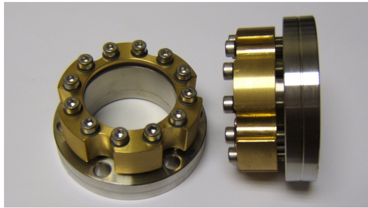
Figure 3.7: Two views of the homemade viewports that were used on both the MOT chamber and deflection chamber to minimise reflections of the laser light coupled into the vacuum system.
