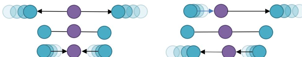
Figure 1.14 - Symmetric (left) and asymmetric (right) stretching modes of  $\text{CO}_2$ <sup>171</sup> Blue: Oxygen, Purple: Carbon
