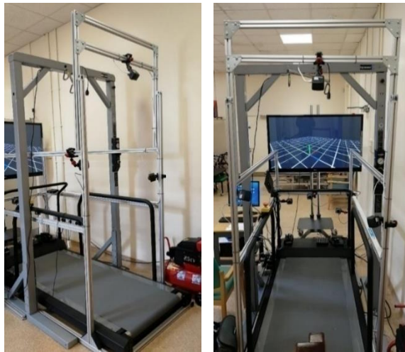
Figure 4.1: six cameras were installed around treadmill.
