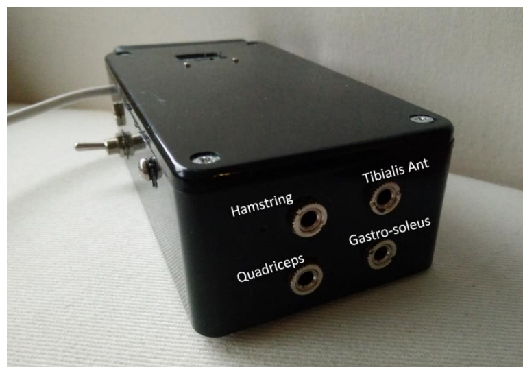
Figure 3.3: The controller box containing the Arduino board with jack sockets.
