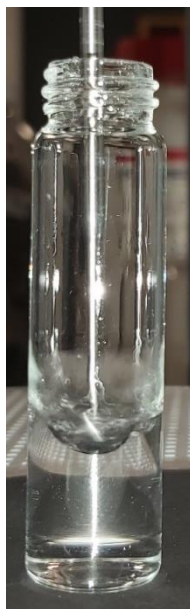
Figure 6:17: Photograph of 8 ml crystalline vial agitated at 2200 RPM using a downward flow three-blade propeller.
