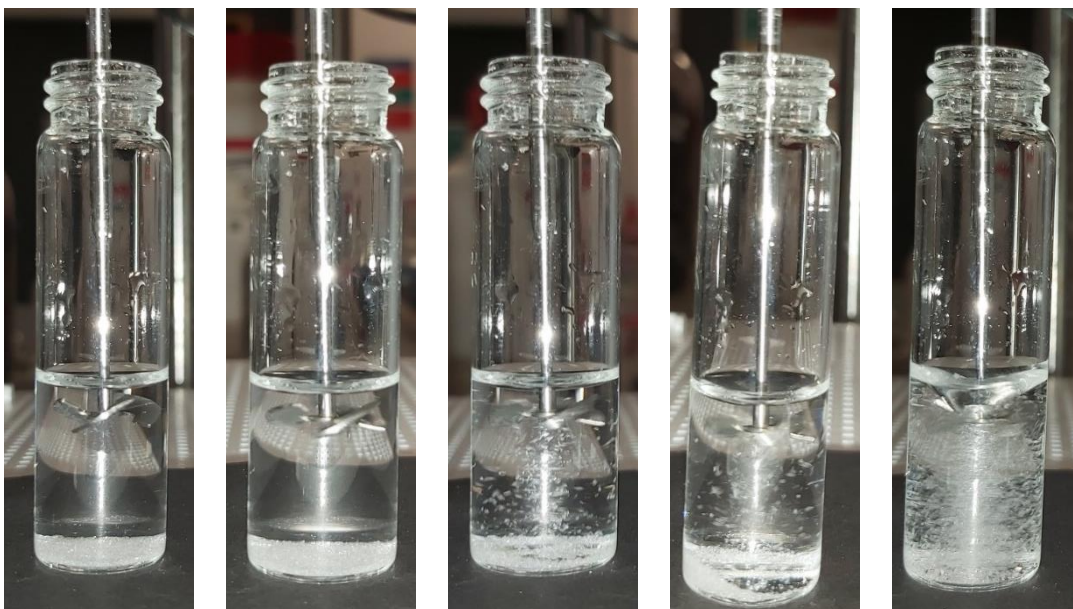
Figure 6:16: Photographs of NaCl suspended in saturated NaCl solution at different agitation rates using a downward flow three-blade propeller (100 RPM, 250 RPM, 500 RPM, 700 RPM, and 1250 RPM; Left to Right)
