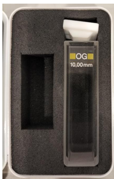
Figure 4:13: Hellma Optical Glass Cuvette (1 cm Path length).
