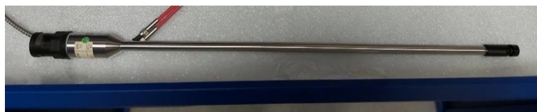
Figure 4:15: Falcata XP 12 Transflectance Probe.
