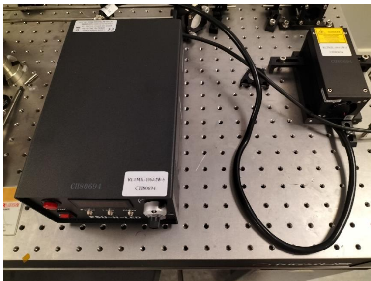
Figure 4:7: 2 W CNI 1064 nm Gaussian Laser.
