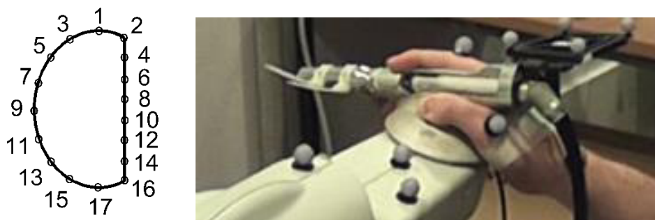
Figure 6.2-12 Tibial shape with numbered points for laser target task (left) Laser Pen attached to end effector (Right)
