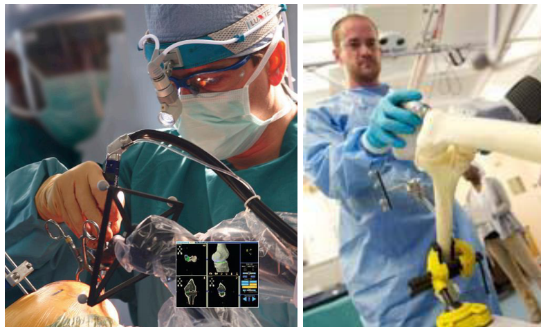
Figure 2.1-4 Image of the change in handle design. TGS (Left) was a 5-degree of freedom robotic arm and held like a pencil. The MAKO RIO (Right) is a 6-degree of freedom robot and held with a spherical prehensile grip.
