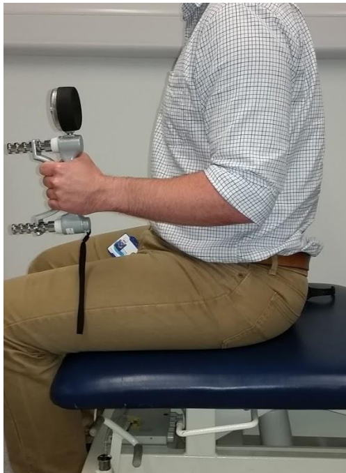
Figure 6.2-3 Example of Dynamometer use for grip strength test. User was sat with the arm at 90 degrees of flexion at the elbow and a neutral shoulder.
