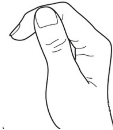
Figure 2.4-5 Lateral Pinch. This pinch has a significantly lower strength than those measured in power grips.
