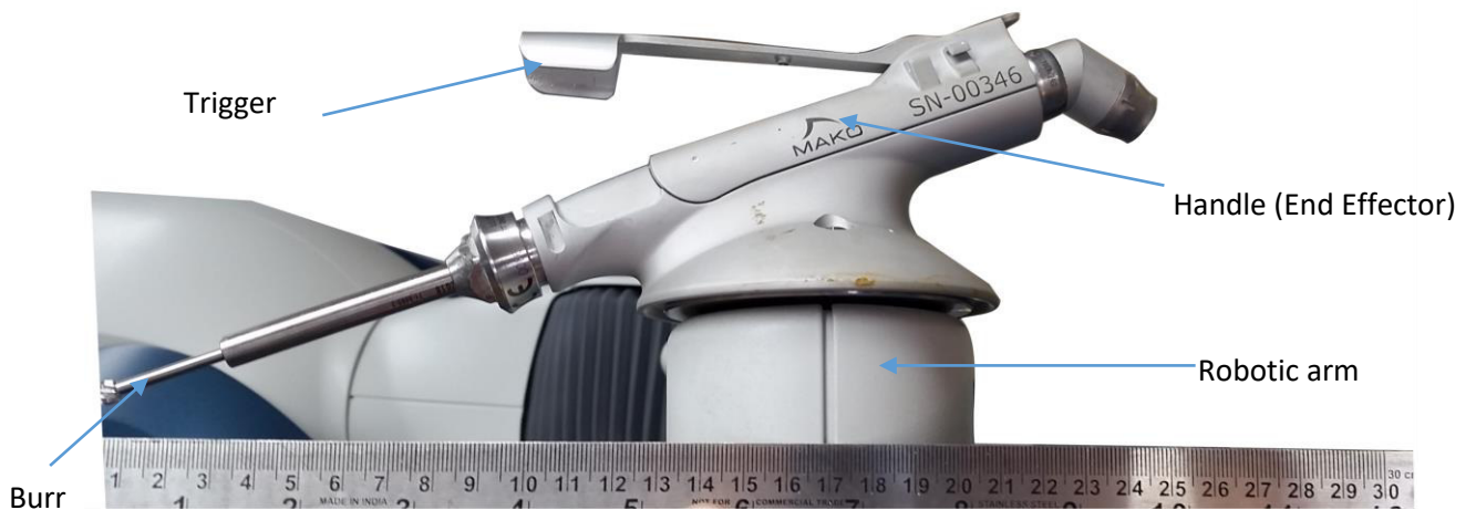
Figure 2.1-5 MAKO RIO Handle (End effector) with scale from cm ruler. This handle/end effector mounts the burr and is manipulated by the surgeon freely moving within a set haptic volume but otherwise restricted to that volume by the robotic arm. The burr is activated through the depression of the trigger and is only position in the haptic volume, if this moves outside of this area the burr is stopped or cannot be activated.
