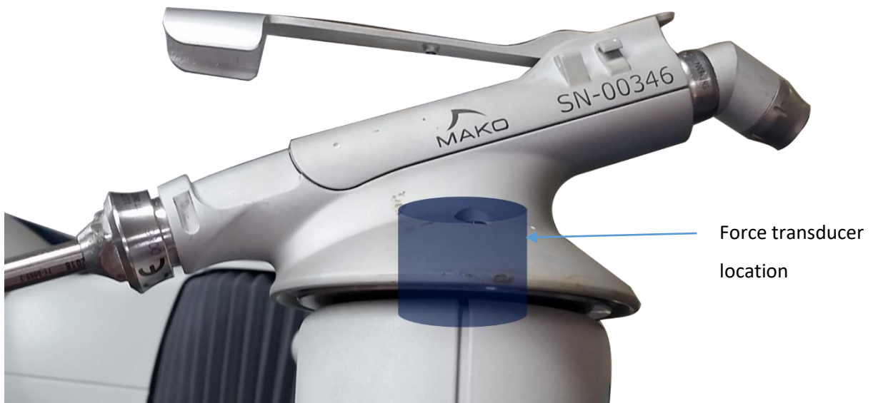
Figure 6.2-11 RIO handle with force transducer location. This measured the force being applied to the handle in all 6 dof. The user was limited to using one hand to ensure that all force was applied through this transducer.
