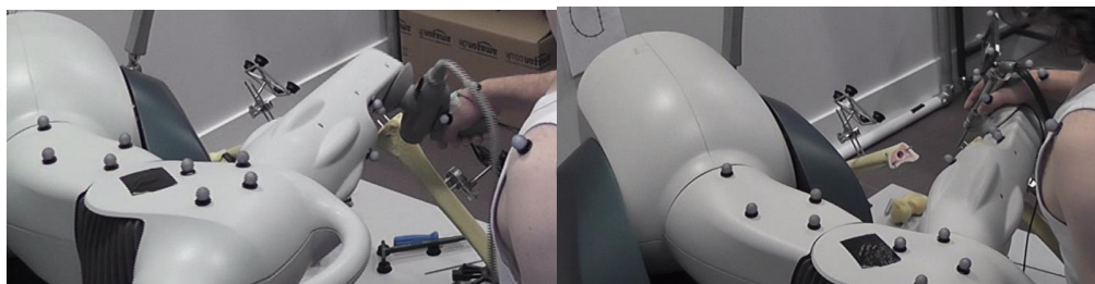
Figure 7.1-3 New prototype (Left) and current handle tibia cut (Right) in use during testing. The new prototype is positioned below and largely blocks the line of sight with the incision. The current handle is attached above and allows a view of the handle.
