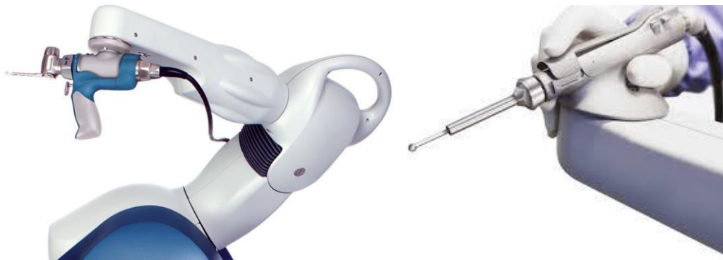
Figure 7.1-1 Images of the finalised handle grip (left) and current end effector (right). The pistol grip results in a power grip, which the current burr is held in a spherical prehensile grip (right).
