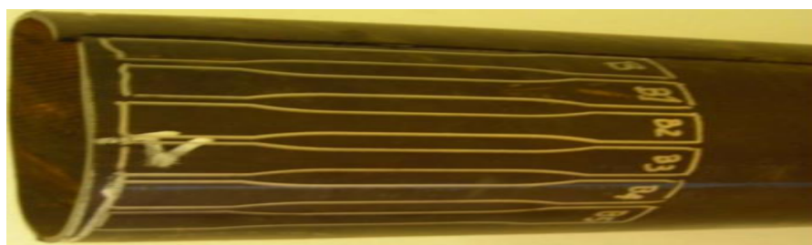
Figure 4-10: External Sheath stress
