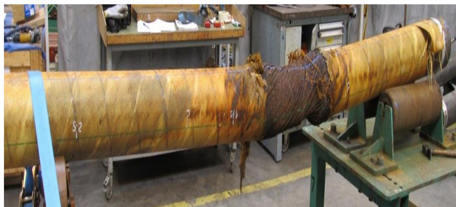
Figure 4-12: Overview of external layers damage
