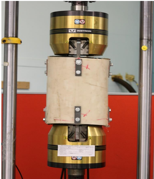
Figure 4-38: Tensile testing arrangement before loading
