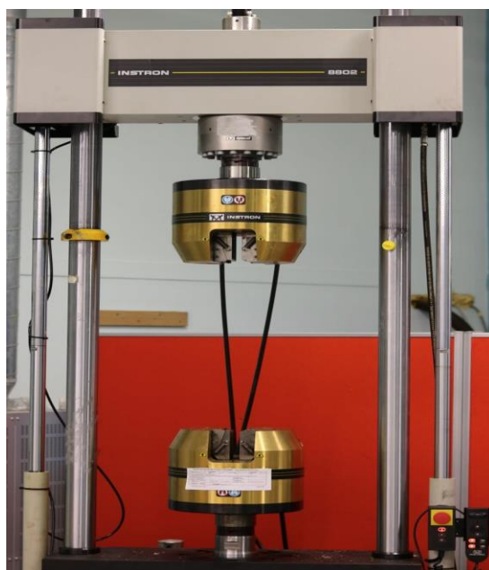
Figure 4-29: Tensile Testing Machine - Instron 8802 (250 kN) Fatigue Test System
