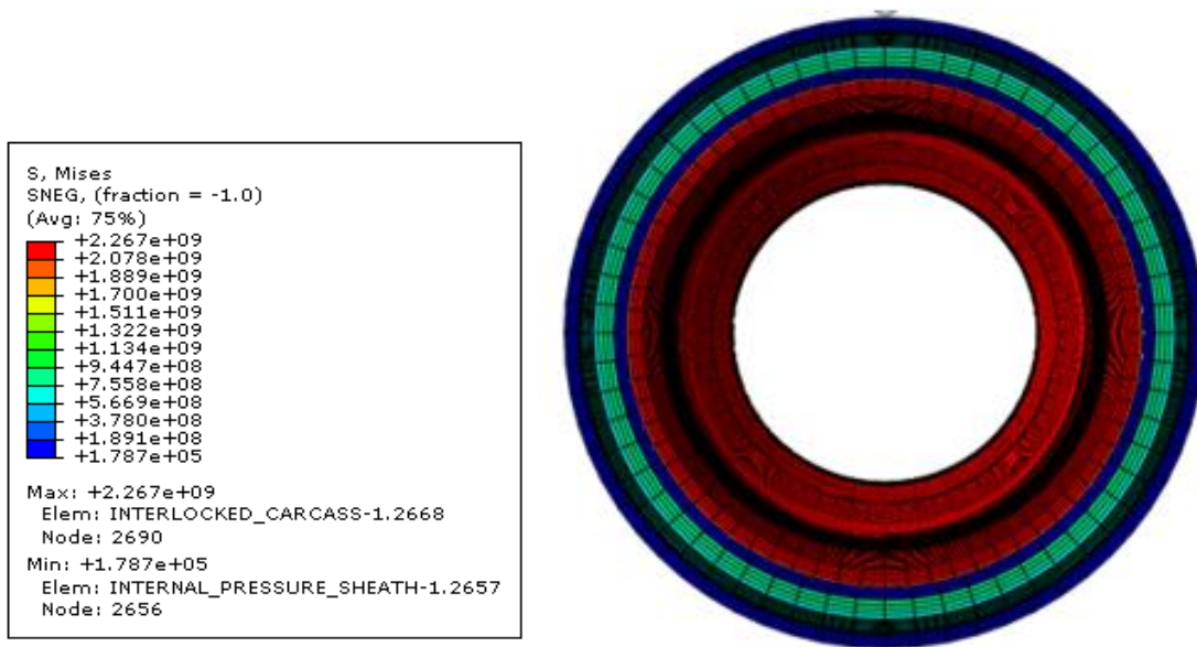
Figure 5-6: Stress Contours under Factory Test Pressure from the end - 3D Model
