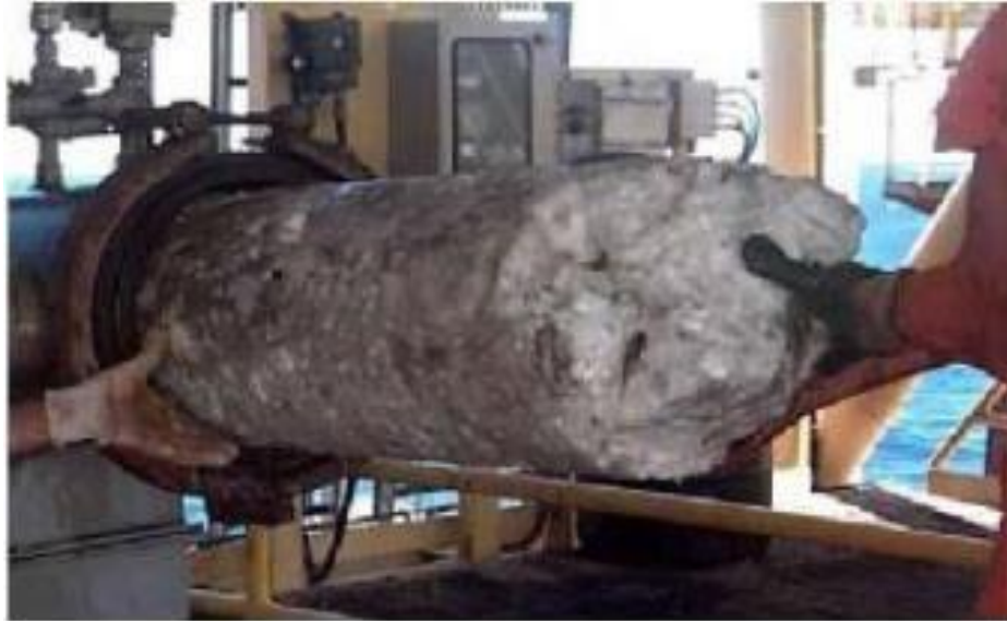
Figure 2-24: Hydrate formation in the natural gas pipeline [33]
