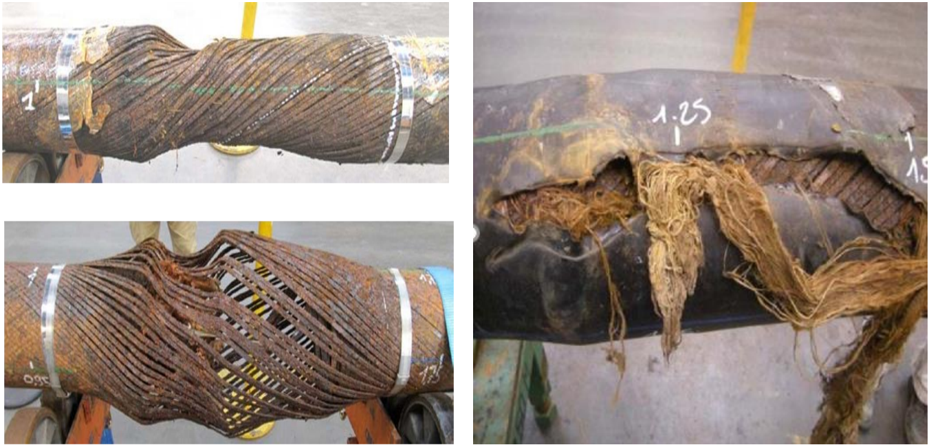
Figure 6-2: Pipe Understudy-Similar deformation with Sample A and B [5]
