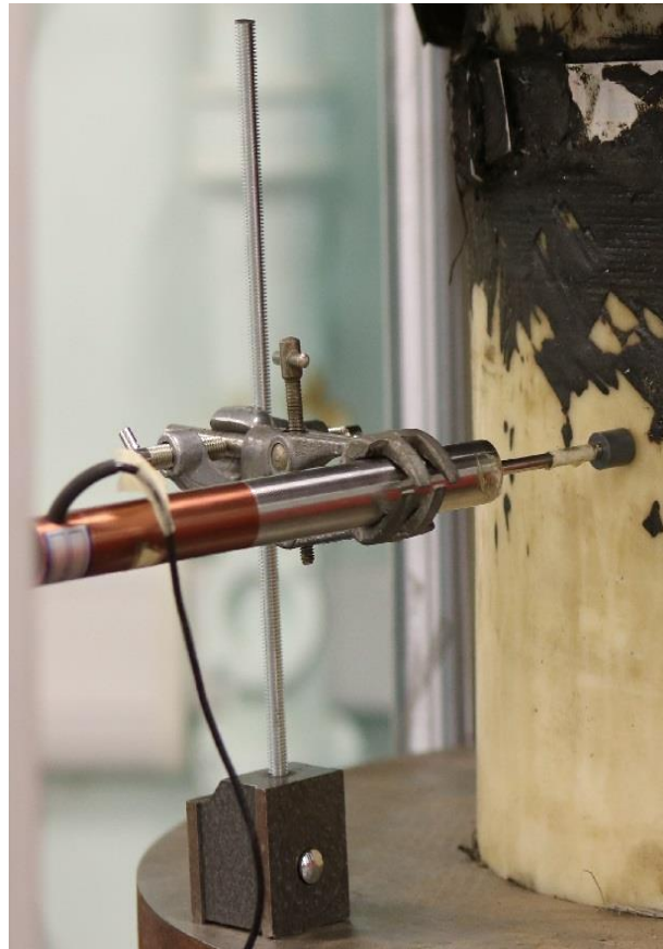
Figure 4-31: RDP Electronic Spring Transducer
