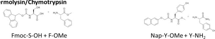
Figure 111 - Full chemical structures of biocatalytic self-assembling aromatic dipeptide amphiphiles in Table 6 . Dotted line represents those used in conjunction with Fmoc-FpY and alkaline phosphatase for co-assembly.
