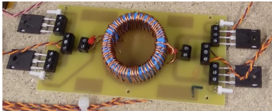
Fig. A.3 DHB converter circuit with nano-crystalline core-based HF transformer.
