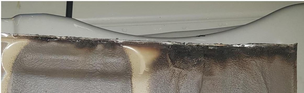
**Figure 60** Cut Edge Quality (Sealant underneath the material)
