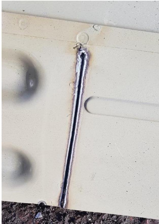
**Figure 61** Quality Obtained after Sealant Removed using Sand Belt.
