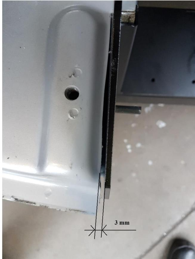
**Figure 2:** Gap between the chassis and the floor pan, (top view of the underbody floor)
