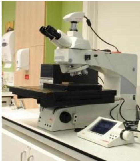
**Figure 19** Leica DM12000 Microscope (AFRC) [165]
