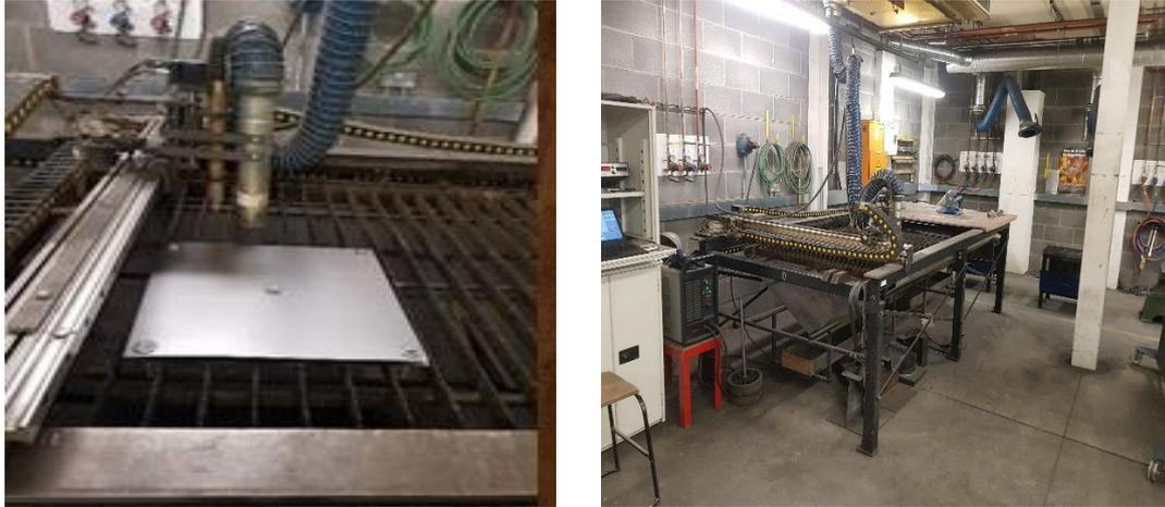
**Figure 16:** CNC Plasma cutter
