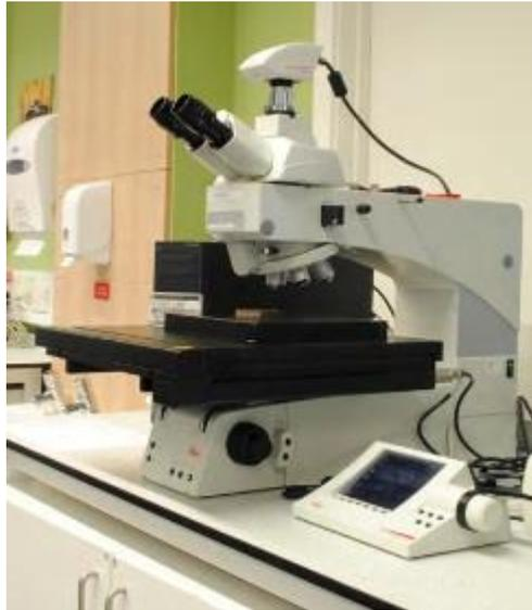
**Figure 19** Leica DM12000 Microscope (AFRC) [165]
