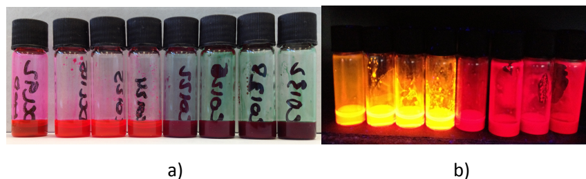
Figure 6-9 T- and Y-shaped oligofluorene BODIPY solutions in toluene. From left to right, T-B1 , T-B2 , T-B3 , T-B4 , Y-B1 , Y-B2 , Y-B3 and Y-B4 . a) Under ambient light. b) Under UV illumination (254 nm).
