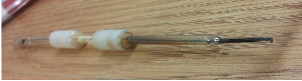
Figure 5.15 Tungsten probe with glass insulator surround
