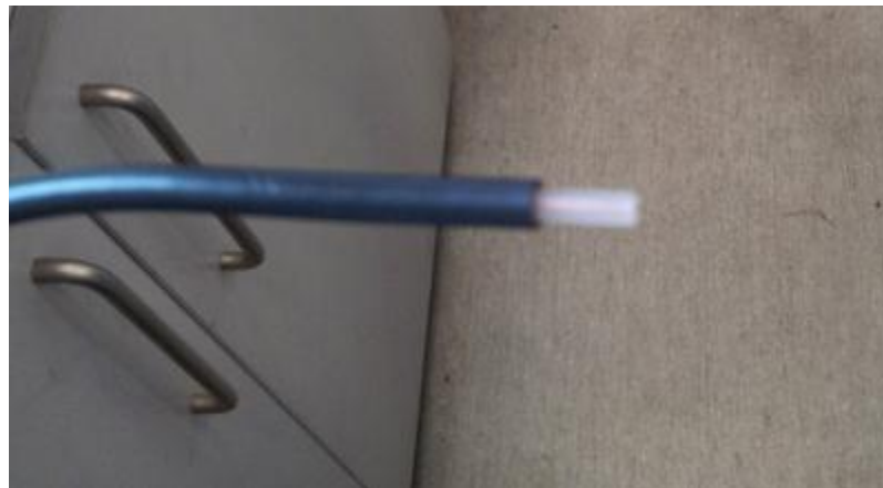
Figure 5.14 Photograph of a simple probe fabricated from co-axial cable
