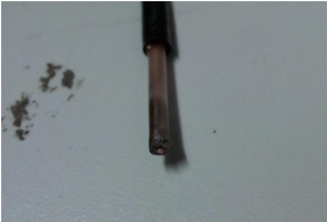
Figure 6.9 Damage caused to Langmuir probe due to thermal heating and electrical arcing
