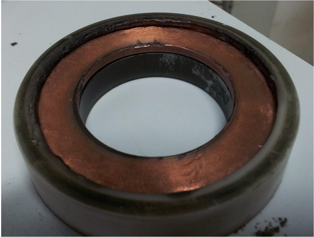
Figure 6.8 Damage caused to Penning trap cathode and insulators due to metal deposition
