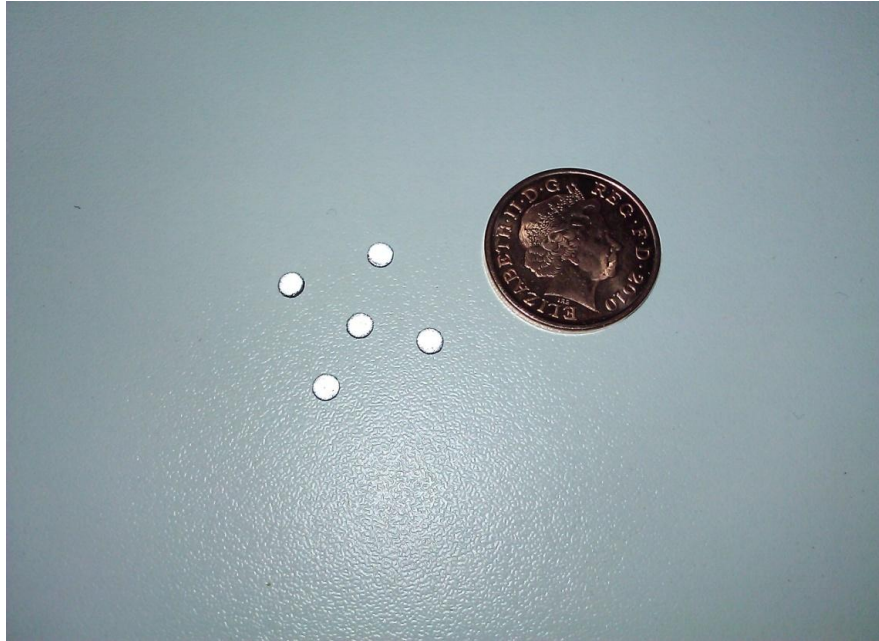
Figure 3.3 – Five 3mm Vicon Reflective Markers with a 1 pence piece for size reference
