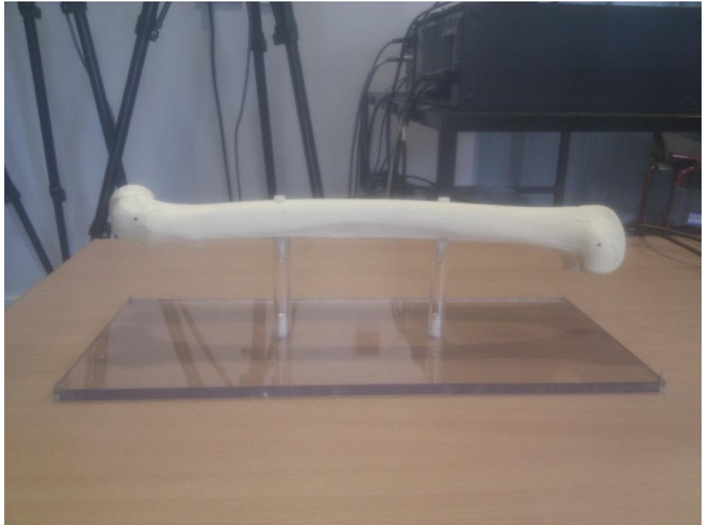
Figure 3.7 Base Plate design with the femur sawbone attached
