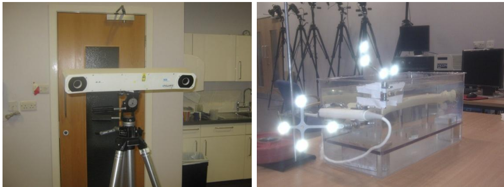
Figure 3.3 & 3.4 Optical Tracking Camera, IR reflecting reference markers
