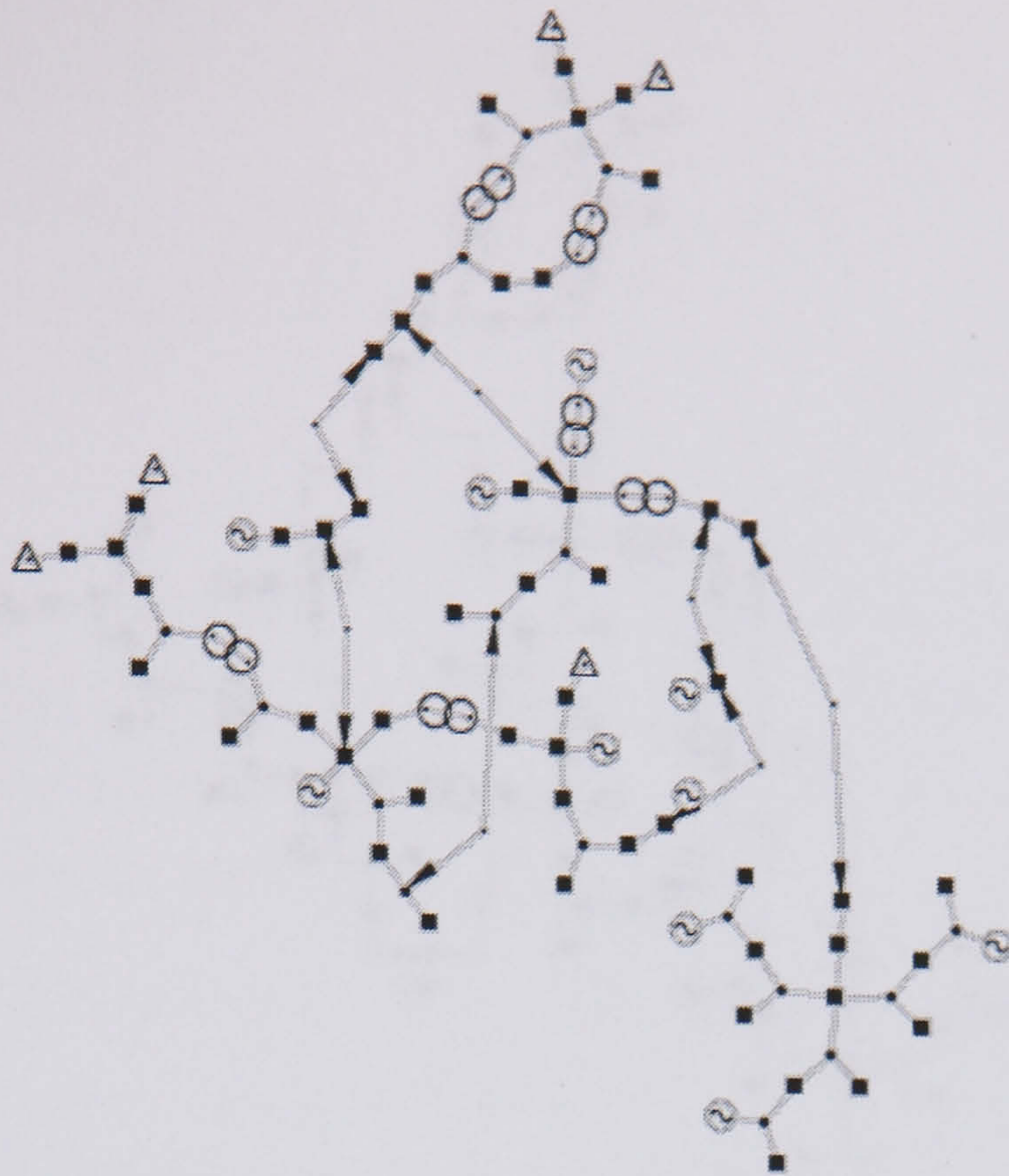
Figure 8.21 Modified Welkin model diagram with power system icons to represent loads, generators, lines and transformers.
