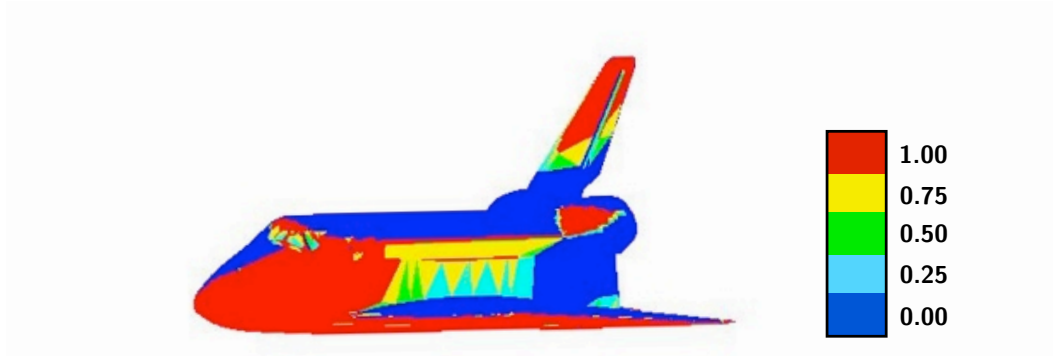
Figure 2.12: Distribution of the visibility ratio per panel over the Space Shuttle Orbiter - The figure depicts the visibility fraction over the tessellated representation of the Space Shuttle Orbiter as result of partial shielding – i.e. when the vehicle operates at 40 degrees angle of attack and 20 degrees sideslip angle.
