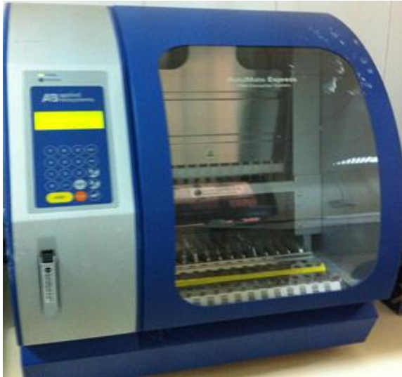
Figure 7-3. AutoMate Express™ DNA Extraction System: The figure show front side of the Robot Extraction System which used for DNA extraction from fired cases.
