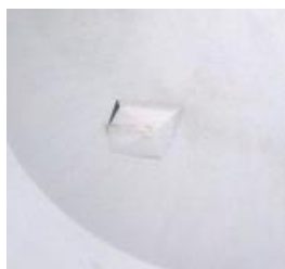
Figure 33. Image of NovO crystal grown under optimised conditions. Growth conditions: 3.5 mg/mL NovO, 20 mM SAH, 0.1 M Mes pH 6.25, 32.73% w/v PEG-4000. Total drop volume: 200 nL.
