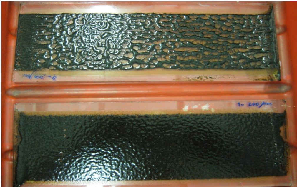
Figure 3-3 polyurethane based material coated with a 200 µm blade
