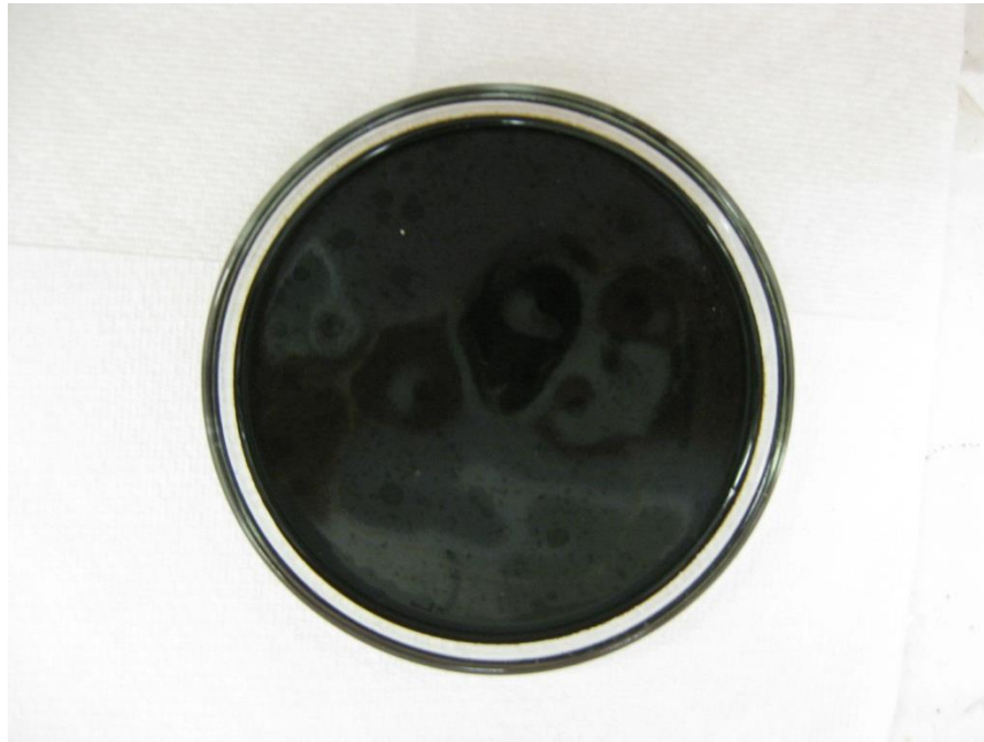
Figure 3-1 polyurethane based material after degassing
