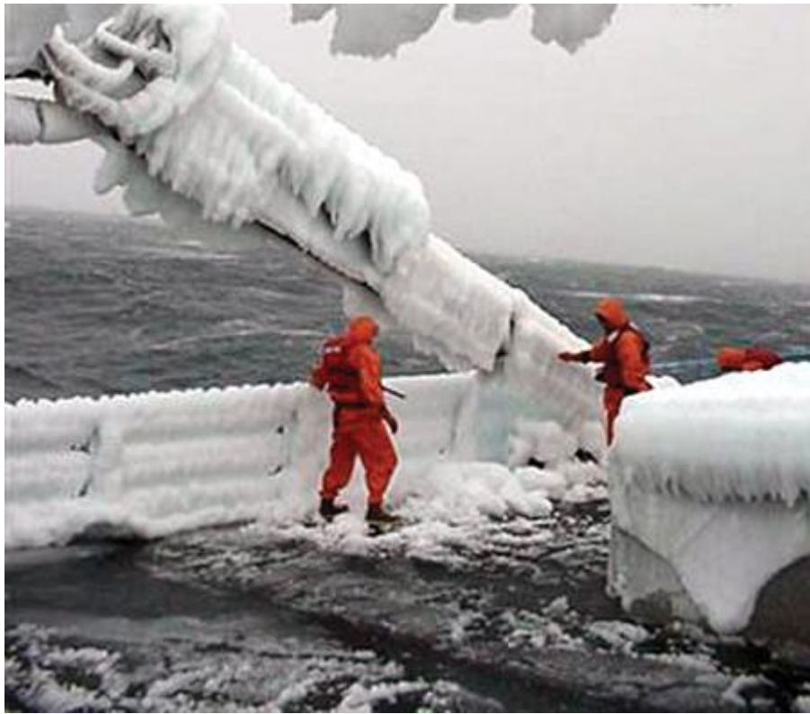
Figure 1-1 Icing on a deck
