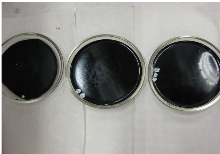
Figure 3-4 polyurethane based material poured without degasing
