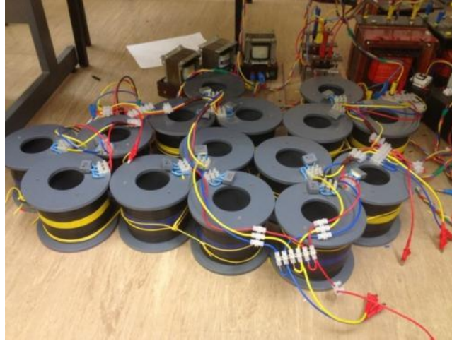
Figure A.19 Wire coils to represent line impedance
