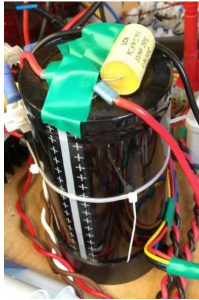
Figure A.10 DC link capacitor
