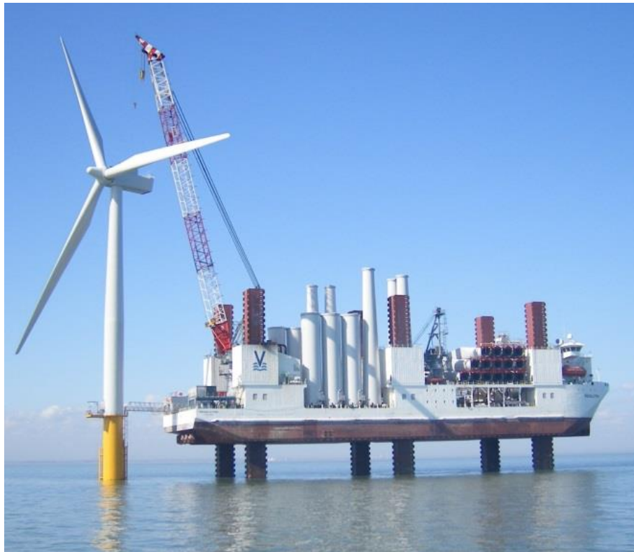
Figure 6.1: Example of a jack-up vessel being used for offshore wind turbine maintenance [6.1].
