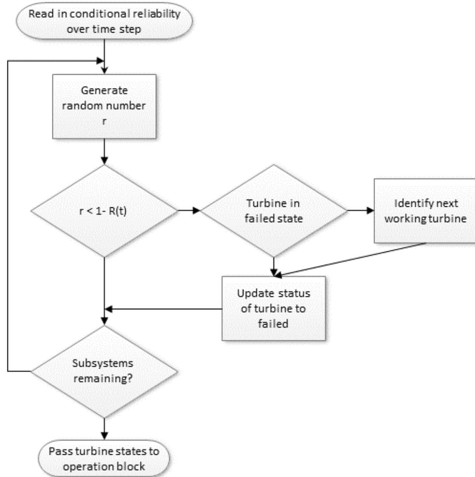
Figure 3.22: Failure simulation process flow chart, identifying preservation of failure rate
