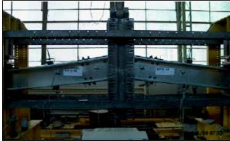
Plate 2.3 Failure of ridge specimens RIS-FB-M (Dubina, 2004b).
