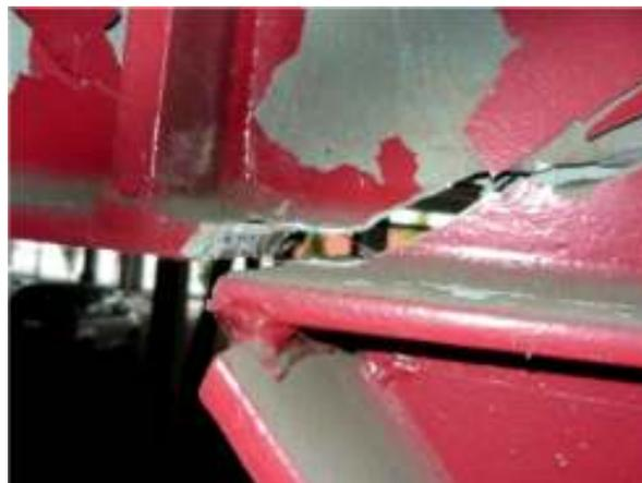
Plate 2.9 Fractured link at lower level EBF (Bruneau et al, 2011)
