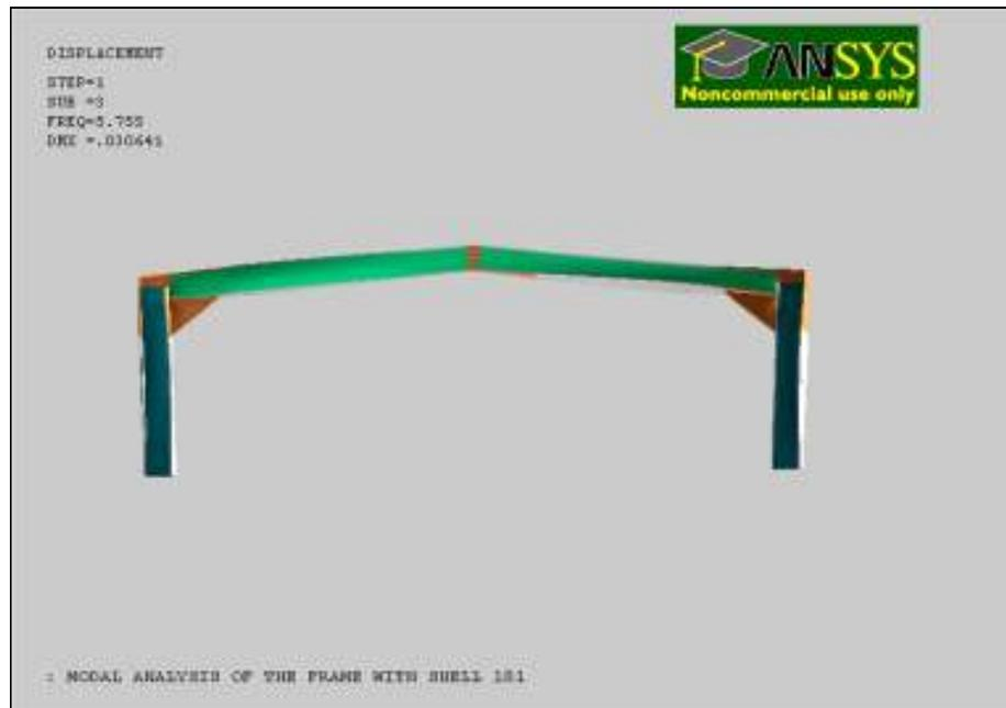
Figure 3.24 Shell mode 3 (Vertical bound and sway)
