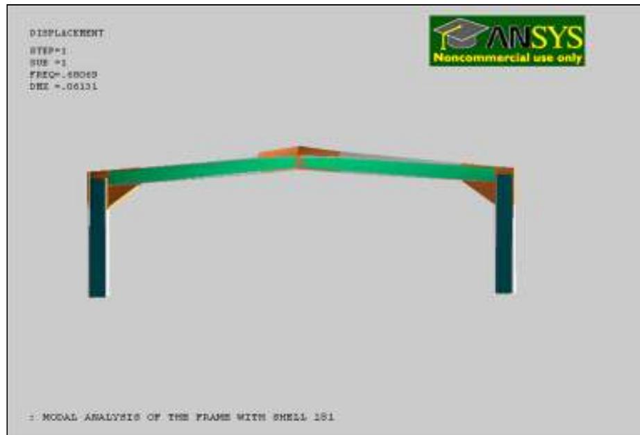
Figure 3.22 Shell mode 1 (Lateral movement)
