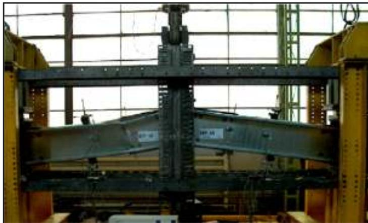
Plate 2.2 Failure of ridge specimens RIP-M (Dubina, 2004b).
