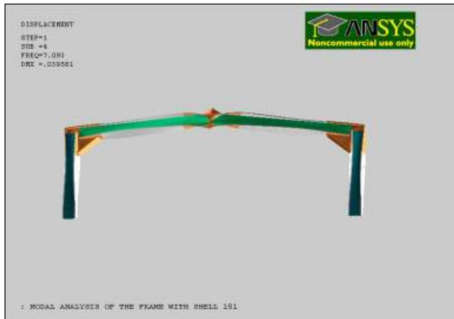
Figure 3.25 Shell mode 4 (Torsional)
