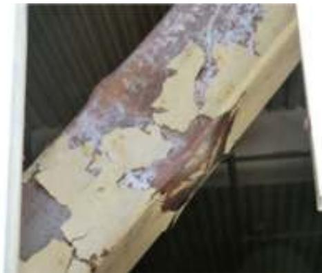
Plate 2.14 Local buckling in square-HSS brace (Midorikawa et al, 2012)
