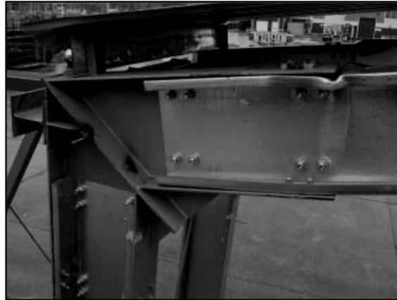
Figure 2.14 C1 frame: local buckling of the left beam connection.
