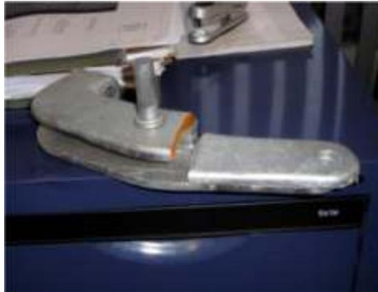
Plate 2.11 Brittle failures of the cast-steel connectors (Clifton, 2011)
