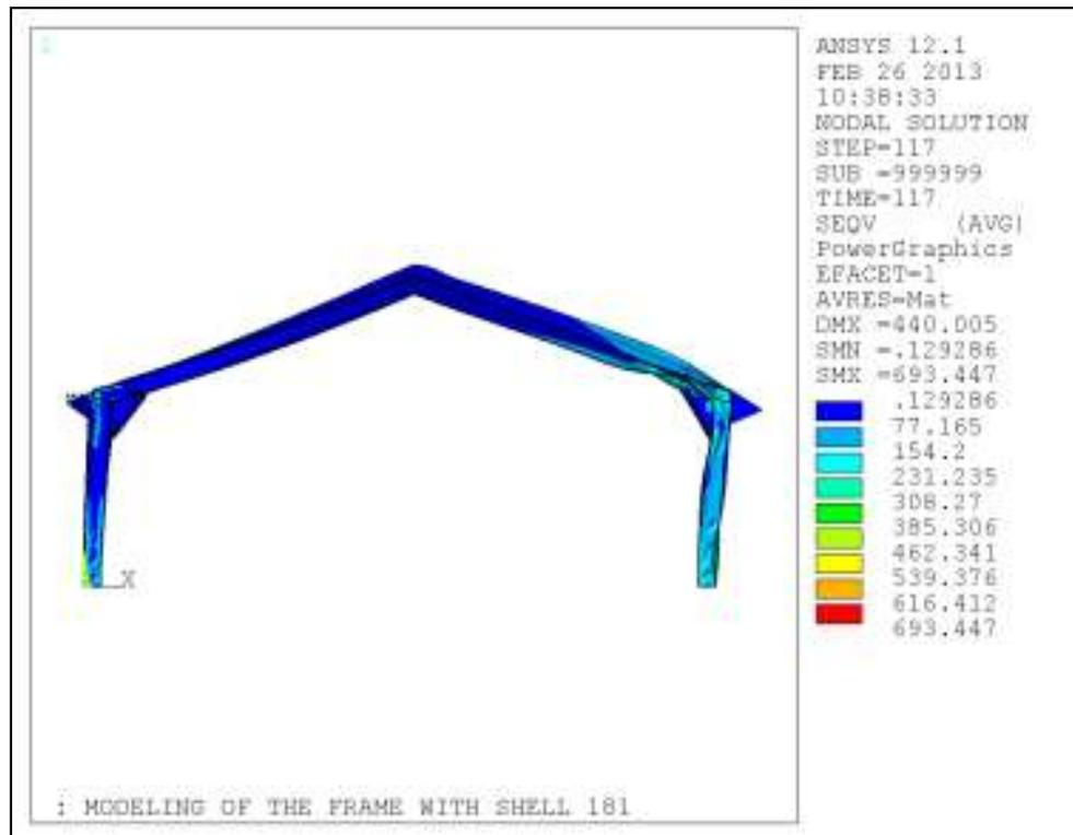
Figure 3.15 Von Mises stress (MPa)
