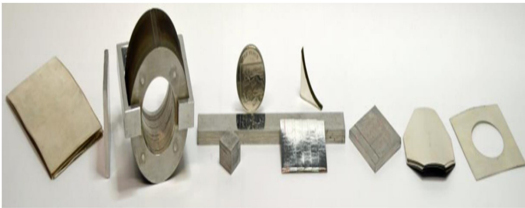
Figure 1-16. HTS tapes pieces and stacks in different shapes and sizes to form composite bulk that has already been produced [63].
