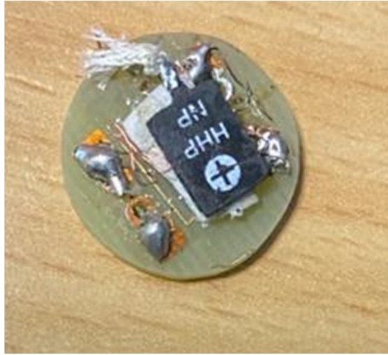
Figure 4-11. Calibrated cryogenic Hall sensor HHP-NP by Arepoc used in this experiment.
