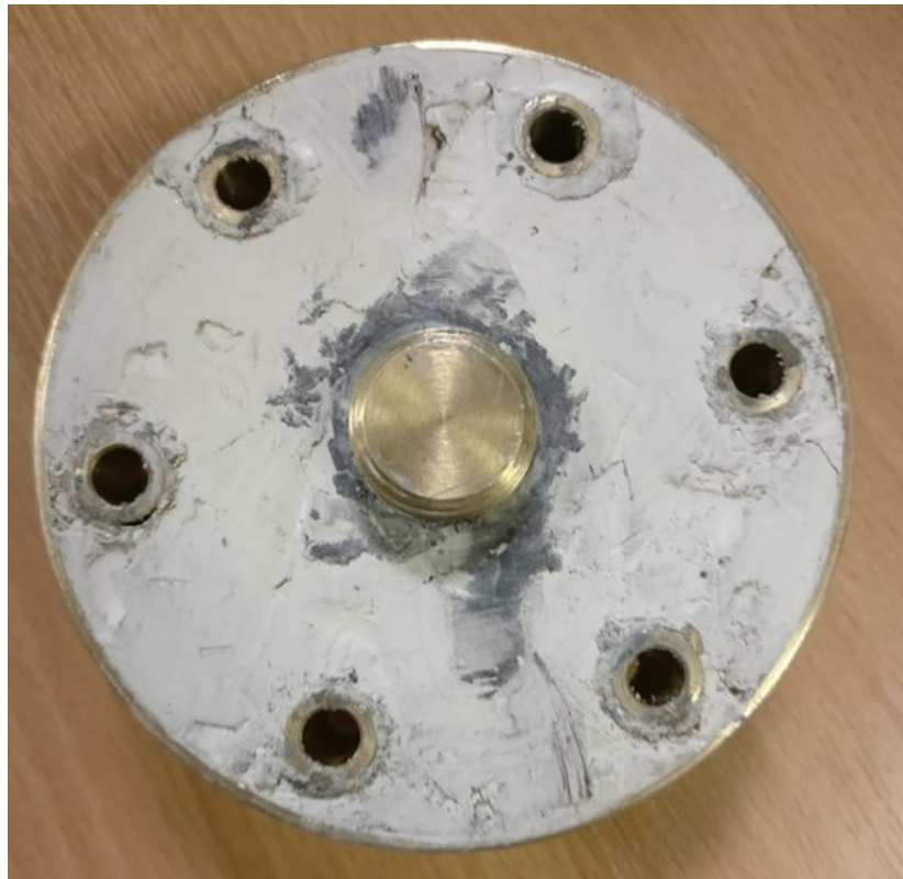
Figure 4-15. Impregnation of the ring magnet sample with a mixture of paraffin wax.
