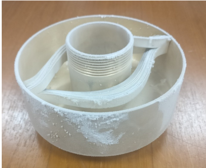
Figure 5-6. Displacement of the ring stack from its original position. Single stack showing an uplift of rings, expansion and pressure at the ends.
