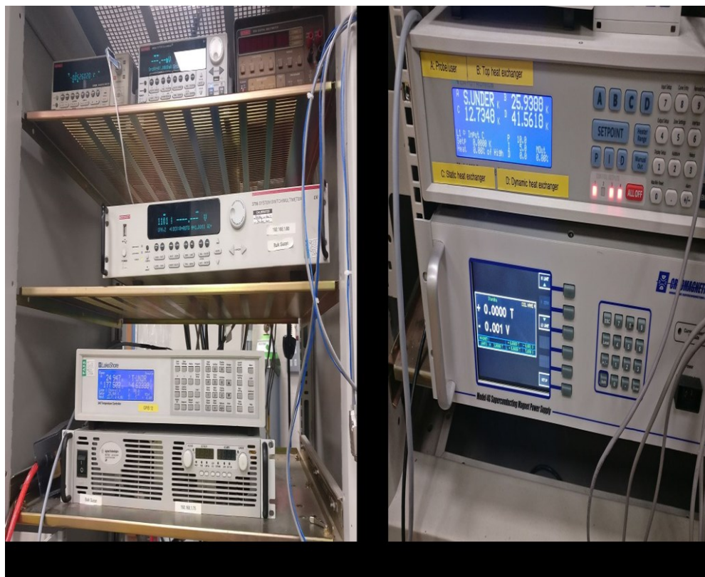
Figure 5-2. a) Data acquisition system, power supplies for sensors, and LakeShore controller for the heater. b) CRYOMAGNETICS power supply and LakeShore temperature controller for monitoring the temperature of the sample and heat exchangers.
