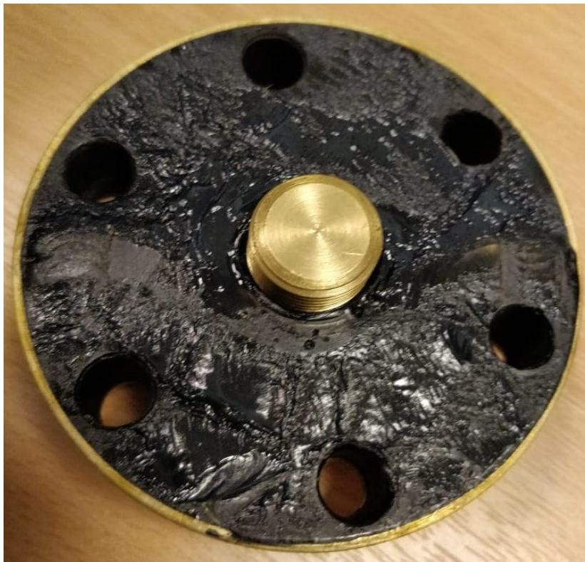
Figure 5-13. Sample holder after drilling holes for cooling purposes. The holes were made to improve the heat dissipation during the cooling down period.
