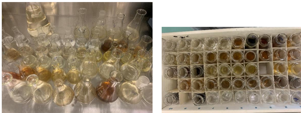
Figure 6.3: Collected fractions by FC showing change in colours between fractions indicating the occurrence of various metabolites in the respective fractions.
