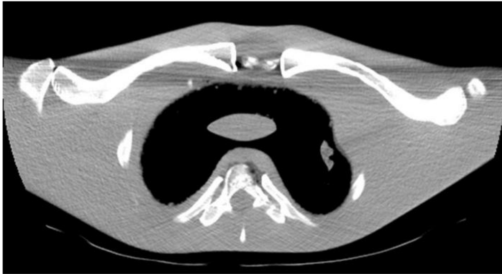
Figure 2.10 CT image of a shoulder phantom shows streaking artefacts by photon starvation [82].
