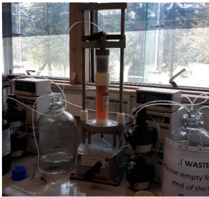
Figure 5.3: MPLC system and flasks used to collect fractions.
