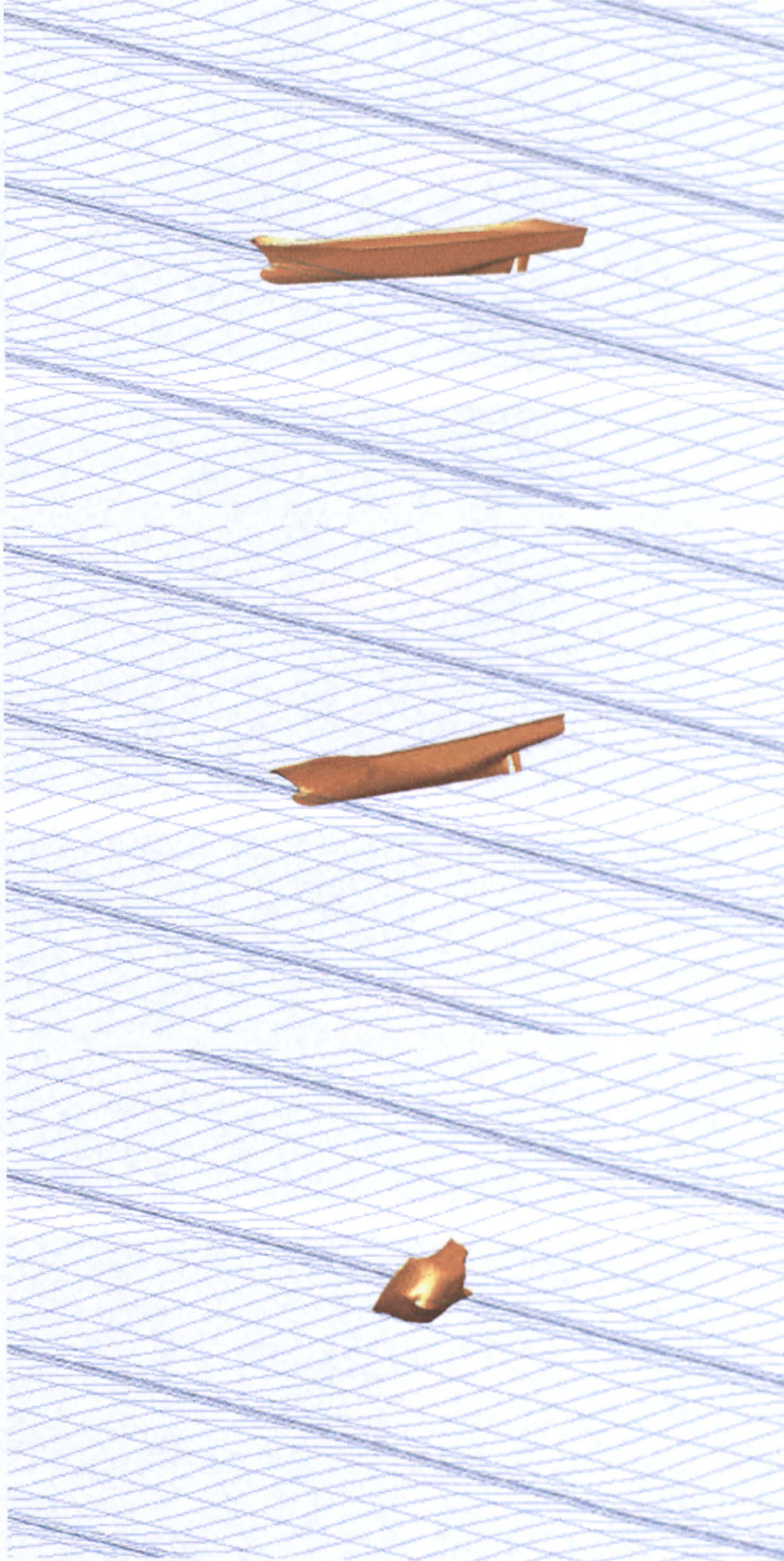
Figure F.6 The sequence of capsize due to broaching for Ship A-2
