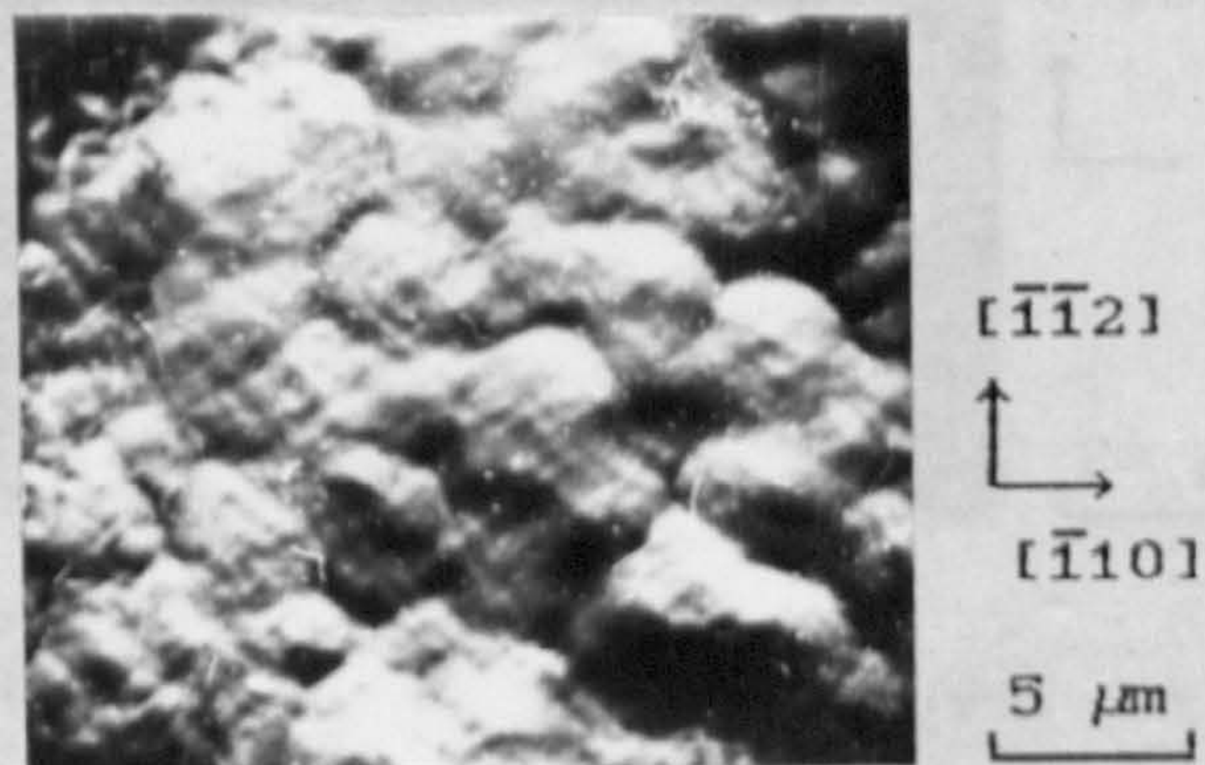
Figure 5.14 (b). A magnified part of the surface shown in (a) revealing tiny, flat hillocks.
