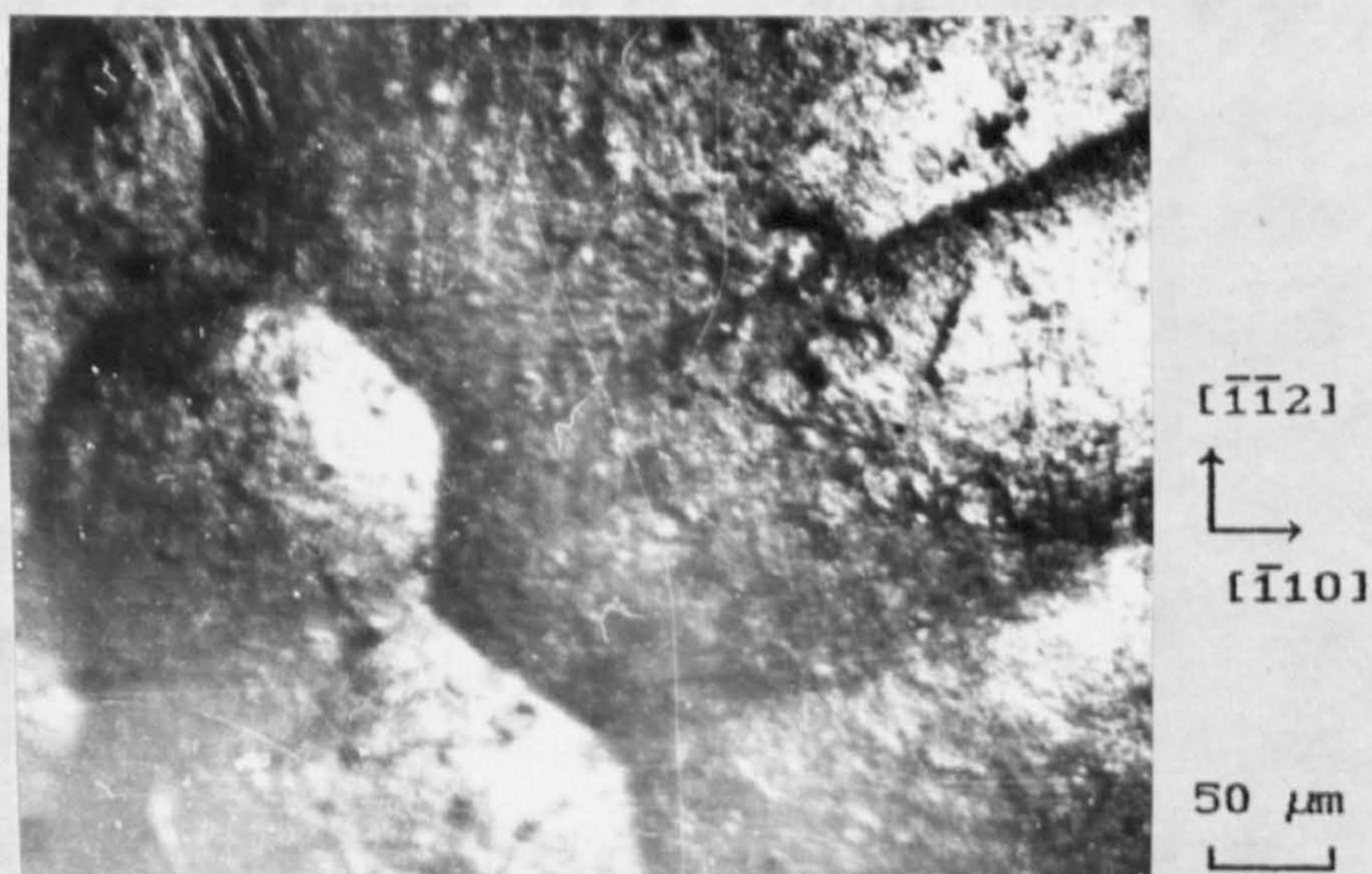
Figure 5.15. Block-like structure observed on the (111) surface of a sodium chlorate crystal grown by solvent evaporation from solution containing 68 ppm of \text{S}_2\text{O}_6^{2-} ions.
